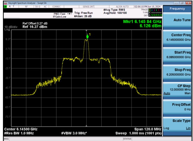
Plot 7-294. SP Power Spectral Density Plot Antenna WF2 (80MHz 802.11ax RU26 (UNII Band 5) – Ch. 39)
