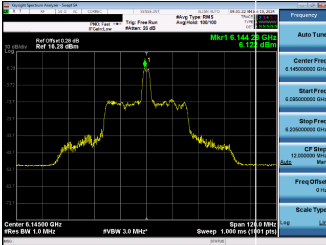
Plot 7-335. SP Power Spectral Density Plot SDM Antenna WF5T (80MHz 802.11ax RU26 (UNII Band 5) – Ch. 39)
