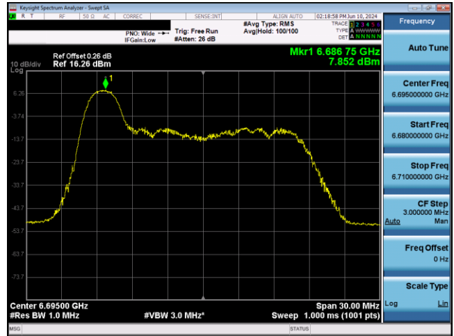
Plot 7-301. SP Power Spectral Density Plot Antenna WF2 (20MHz 802.11ax RU26 (UNII Band 7) – Ch. 149)
