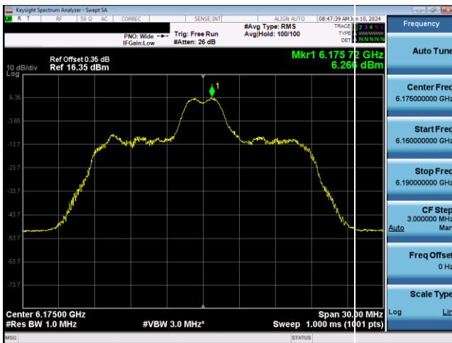
Plot 7-319. SP Power Spectral Density Plot SDM Antenna WF5T (20MHz 802.11ax RU26 (UNII Band 5) – Ch. 45)
