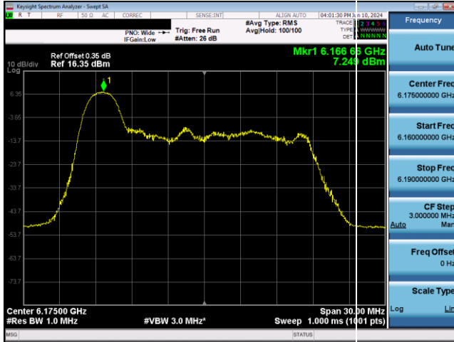
Plot 7-318. SP Power Spectral Density Plot SDM Antenna WF2 (20MHz 802.11ax RU26 (UNII Band 5) – Ch. 45)
