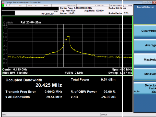
Plot 7-235. 26dB & 99% Bandwidth Plot Antenna WF2 VLP (160MHz 802.11ax RU26 (UNII Band 5) – Ch. 47)
