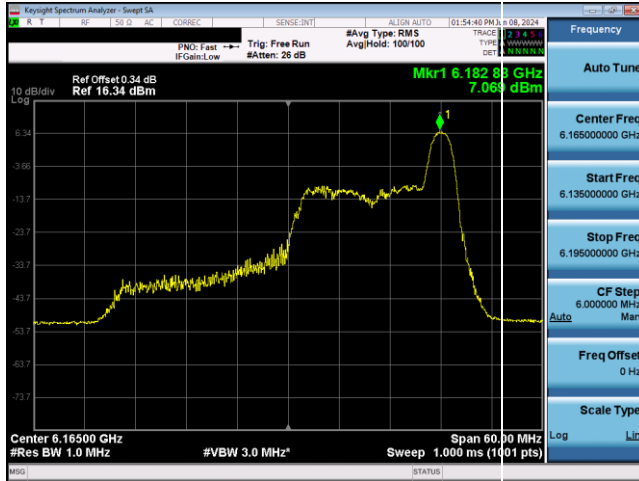
Plot 7-259. SP Power Spectral Density Plot Antenna WF5T (40MHz 802.11ax RU26 (UNII Band 5) - Ch. 43)
