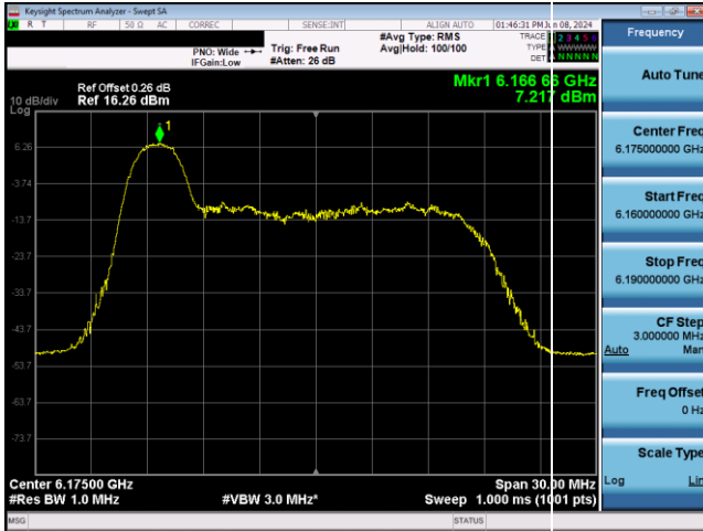
Plot 7-253. SP Power Spectral Density Plot Antenna WF5T (20MHz 802.11ax RU26 (UNII Band 5) – Ch. 45)
