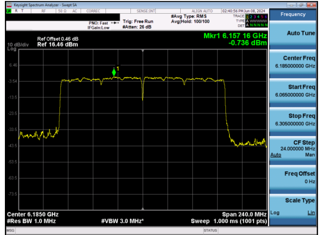
Plot 7-268. SP Power Spectral Density Plot Antenna WF5T (160MHz 802.11ax RU996x2 (UNII Band 5) – Ch. 47)
