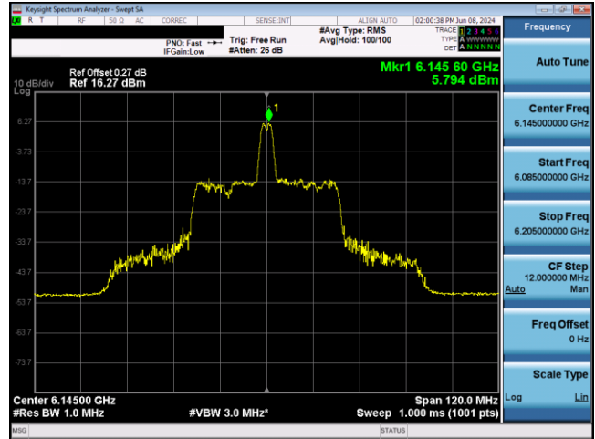
Plot 7-262. SP Power Spectral Density Plot Antenna WF5T (80MHz 802.11ax RU26 (UNII Band 5) - Ch. 39)
