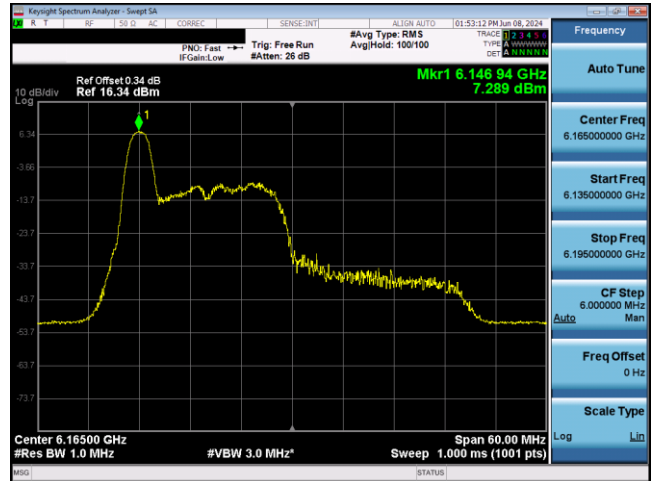
Plot 7-257. SP Power Spectral Density Plot Antenna WF5T (40MHz 802.11ax RU26 (UNII Band 5) – Ch. 43)
