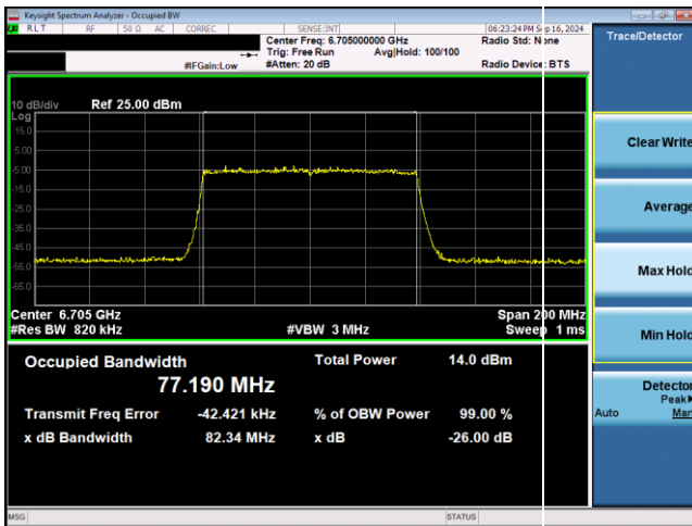
Plot 7-218. 26dB & 99% Bandwidth Plot Antenna WF5T VLP (80MHz 802.11ax RU996 (UNII Band 7) – Ch. 151)
