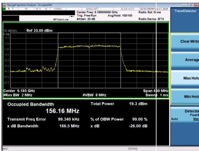
Plot 7-207. 26dB & 99% Bandwidth Plot Antenna WF5T VLP (160MHz 802.11ax RU996x2 (UNII Band 5) – Ch. 47)
