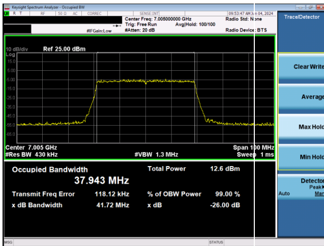
Plot 7-120. 26dB & 99% Bandwidth Plot Antenna WF5T LPI (40MHz 802.11ax RU484 (UNII Band 8) – Ch. 211)
