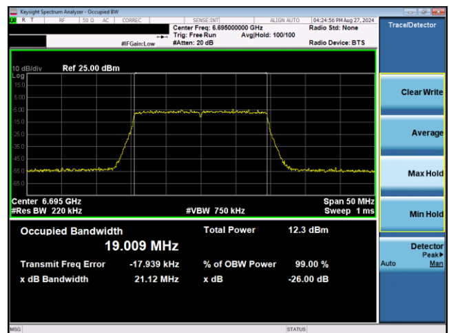
Plot 7-164. 26dB & 99% Bandwidth Plot Antenna WF2 LPI (20MHz 802.11ax RU242 (UNII Band 7) – Ch. 149)
