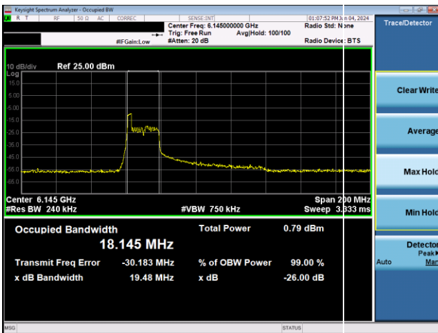
Plot 7-137. 26dB & 99% Bandwidth Plot Antenna WF2 LPI (80MHz 802.11ax RU26 (UNII Band 5) – Ch. 39)
