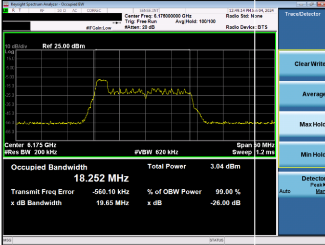
Plot 7-129. 26dB & 99% Bandwidth Plot Antenna WF2 LPI (20MHz 802.11ax RU26 (UNII Band 5) – Ch. 45)
