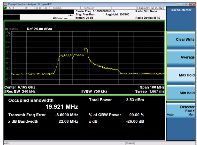
Plot 7-134. 26dB & 99% Bandwidth Plot Antenna WF2 LPI (40MHz 802.11ax RU26 (UNII Band 5) – Ch. 43)
