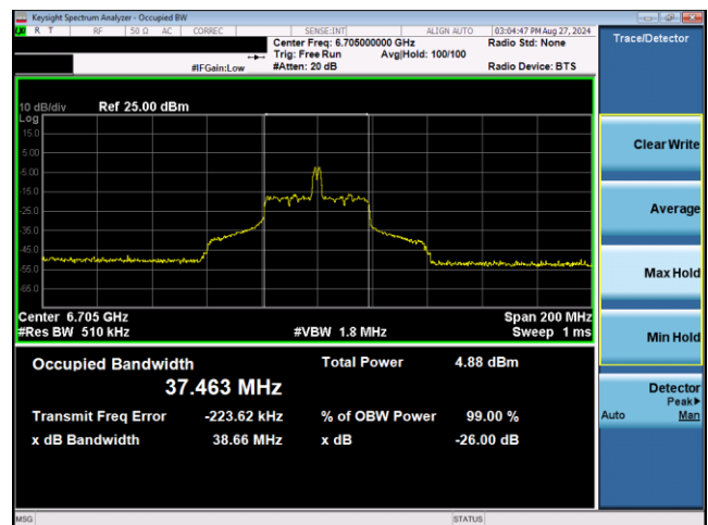
Plot 7-106. 26dB & 99% Bandwidth Plot Antenna WF5T LPI (80MHz 802.11ax RU26 (UNII Band 7) – Ch. 151)
