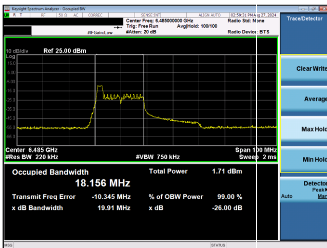
Plot 7-85. 26dB & 99% Bandwidth Plot Antenna WF5T LPI (40MHz 802.11ax RU26 (UNII Band 6) – Ch. 107)
