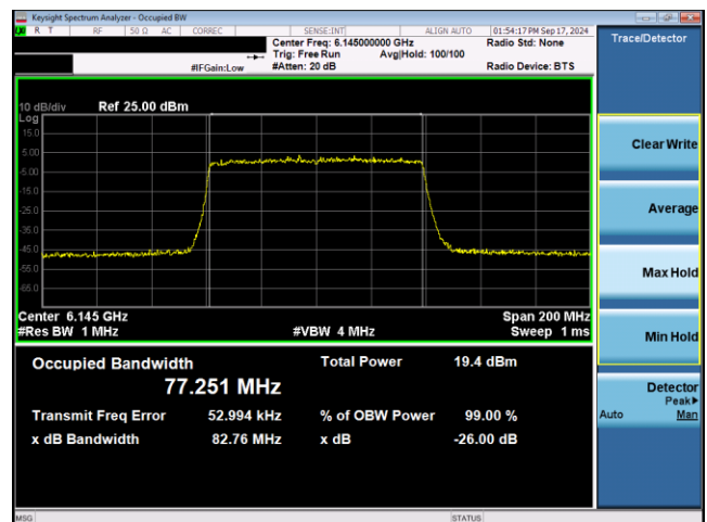
Plot 7-76. 26dB & 99% Bandwidth Plot Antenna WF5T LPI (80MHz 802.11ax RU996 (UNII Band 5) – Ch. 39)
