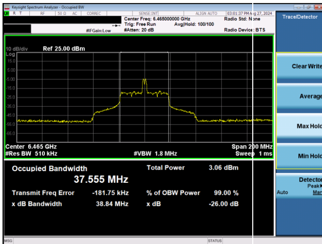
Plot 7-90. 26dB & 99% Bandwidth Plot Antenna WF5T LPI (80MHz 802.11ax RU26 (UNII Band 6) – Ch. 103)
