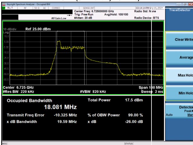
Plot 7-53. 26dB & 99% Bandwidth Plot Antenna WF2 SP (40MHz 802.11ax RU26 (UNII Band 7) – Ch. 155)
