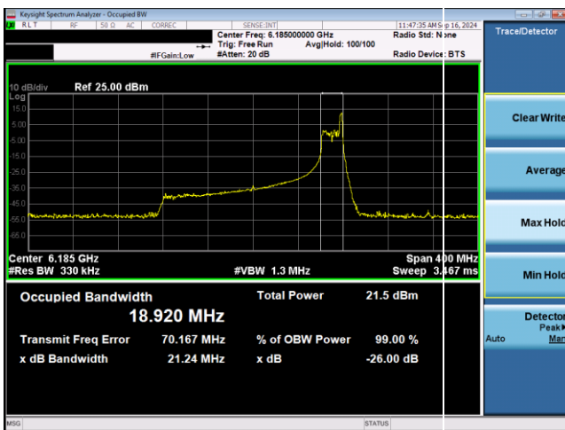
Plot 7-15. 26dB & 99% Bandwidth Plot Antenna WF5T SP (160MHz 802.11ax RU26 (UNII Band 5) – Ch. 47)
