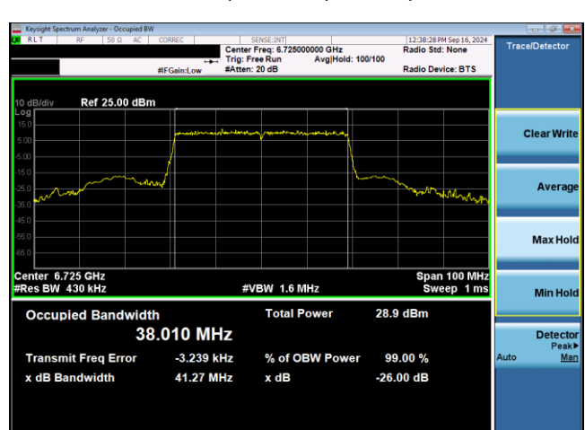
Plot 7-24. 26dB & 99% Bandwidth Plot Antenna WF5T SP (40MHz 802.11ax RU484 (UNII Band 7) – Ch. 155)
