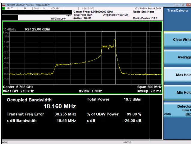
Plot 7-27. 26dB & 99% Bandwidth Plot Antenna WF5T SP (80MHz 802.11ax RU26 (UNII Band 7) – Ch. 151)
