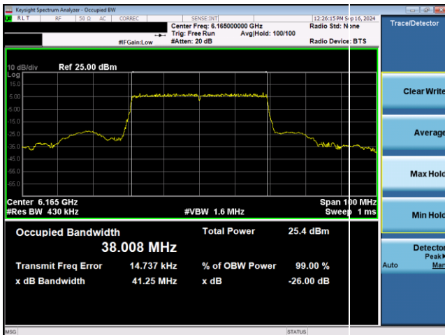
Plot 7-8. 26dB & 99% Bandwidth Plot Antenna WF5T SP (40MHz 802.11ax RU484 (UNII Band 5) – Ch. 43)
