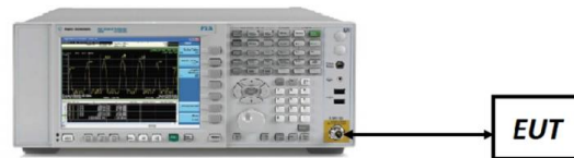
Figure 7-7. Test Instrument & Measurement Setup
