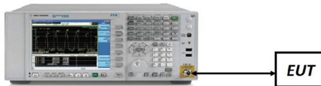
Figure 7-4. Test Instrument & Measurement Setup
