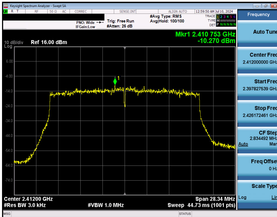
Plot 7-152. Power Spectral Density Plot CDD Antenna WF7 (802.11ax (SU - 2.4GHz) – Ch. 1) – MCS4
