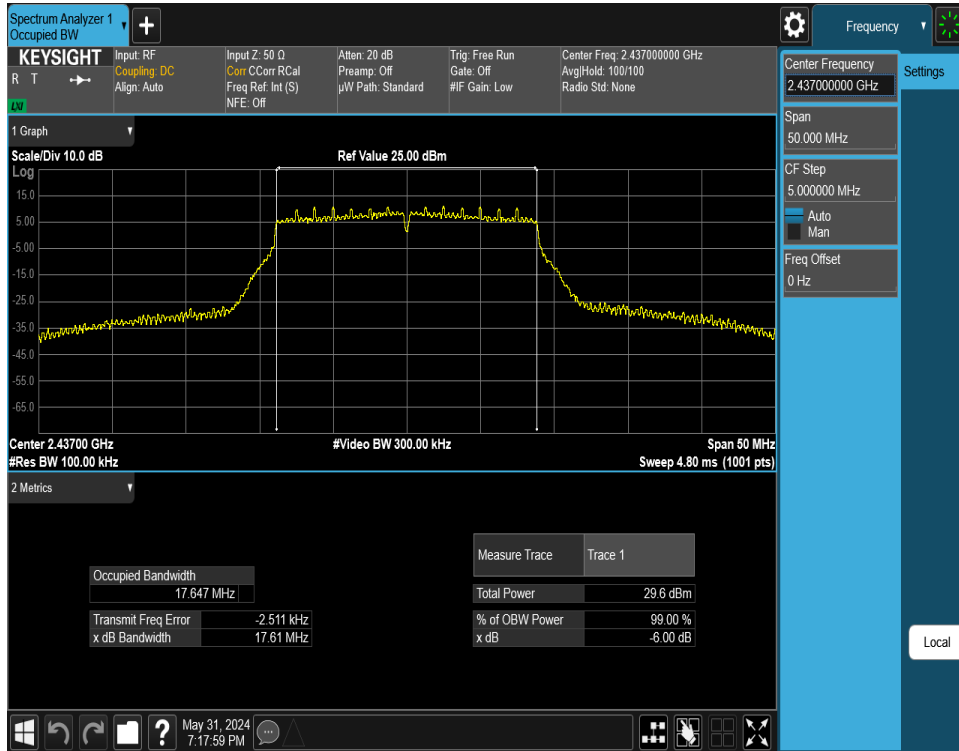
Plot 7-35. 6 dB BW and 99% OBW Plot Antenna WF7 (802.11n (2.4GHz) – Ch. 6) – MCS2
