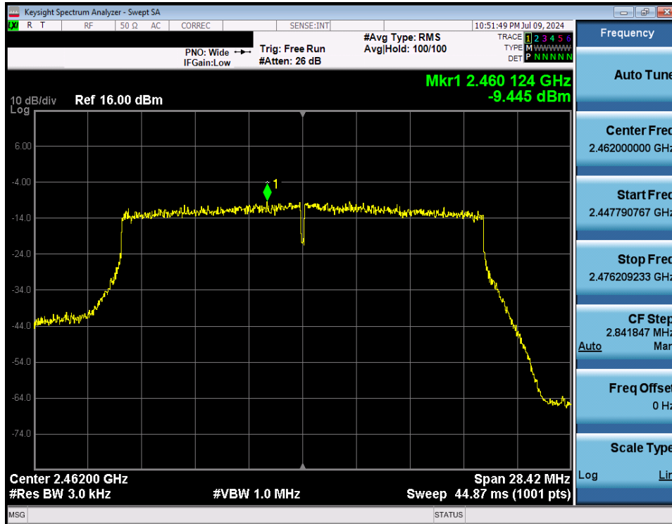
Plot 7-69. Power Spectral Density Plot Antenna WF8 (802.11ax (SU - 2.4GHz) – Ch. 11) – MCS2
