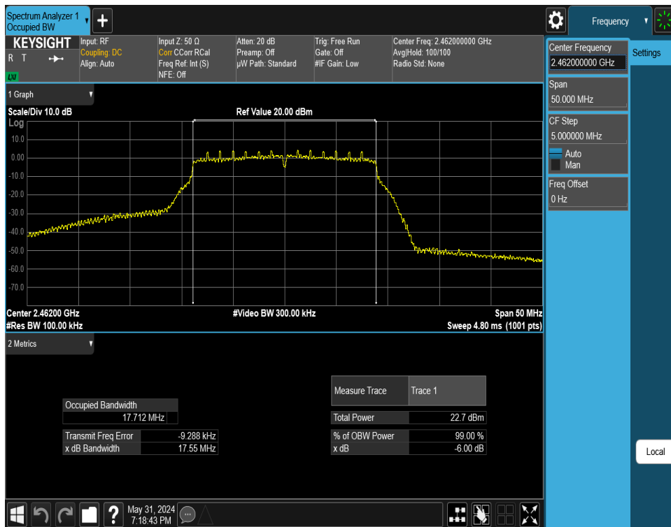
Plot 7-36. 6 dB BW and 99% OBW Plot Antenna WF7 (802.11n (2.4GHz) – Ch. 11) – MCS2
