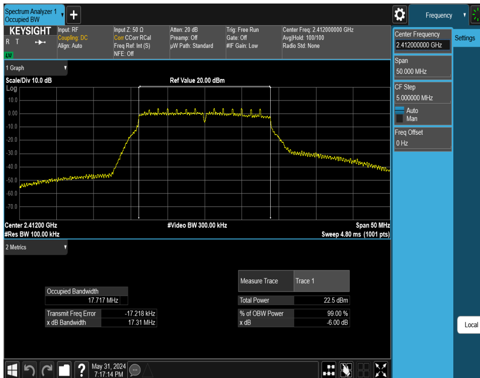
Plot 7-34. 6 dB BW and 99% OBW Plot Antenna WF7 (802.11n (2.4GHz) – Ch. 1) – MCS2
