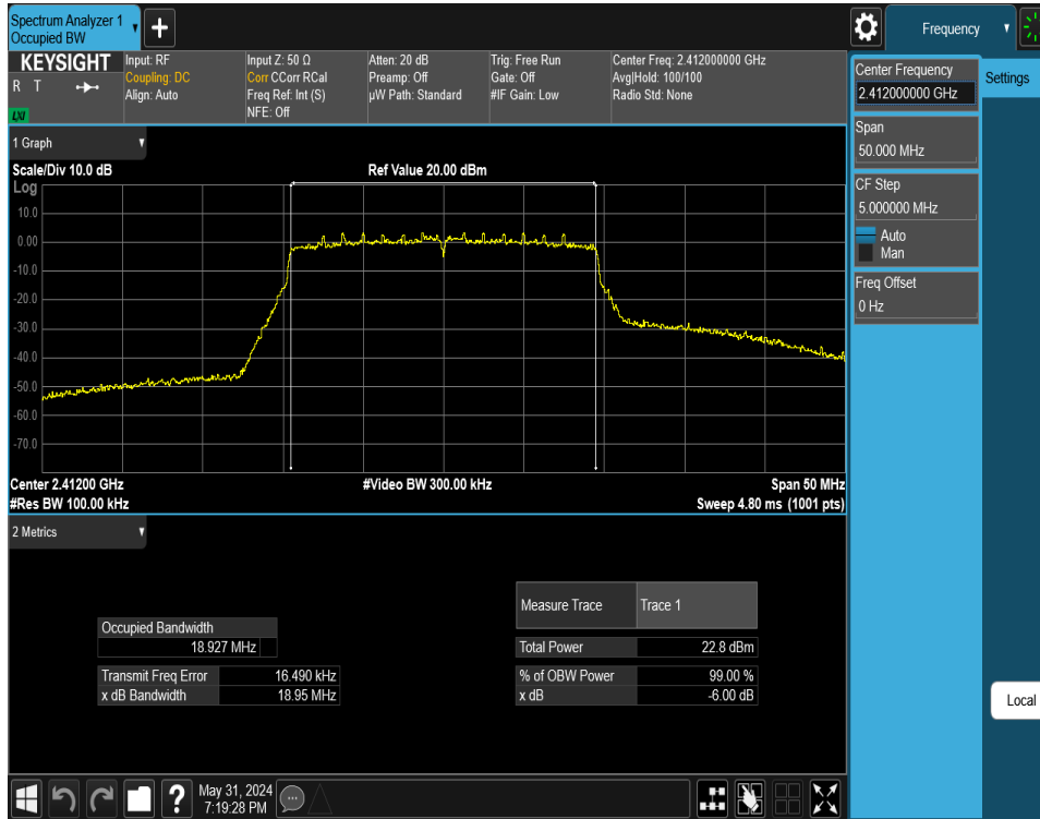
Plot 7-37. 6 dB BW and 99% OBW Plot Antenna WF7 (802.11ax (SU - 2.4GHz) – Ch. 1) – MCS2
