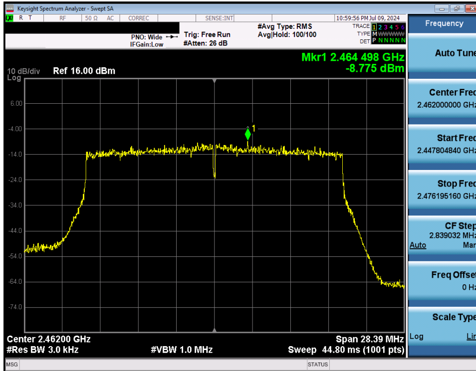
Plot 7-78. Power Spectral Density Plot Antenna WF8 (802.11ax (SU - 2.4GHz) – Ch. 11) – MCS4
