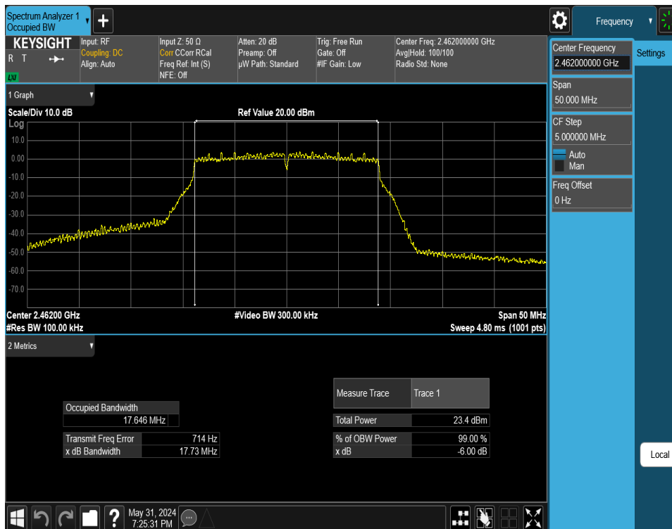
Plot 7-45. 6 dB BW and 99% OBW Plot Antenna WF7 (802.11n (2.4GHz) – Ch. 11) – MCS4
