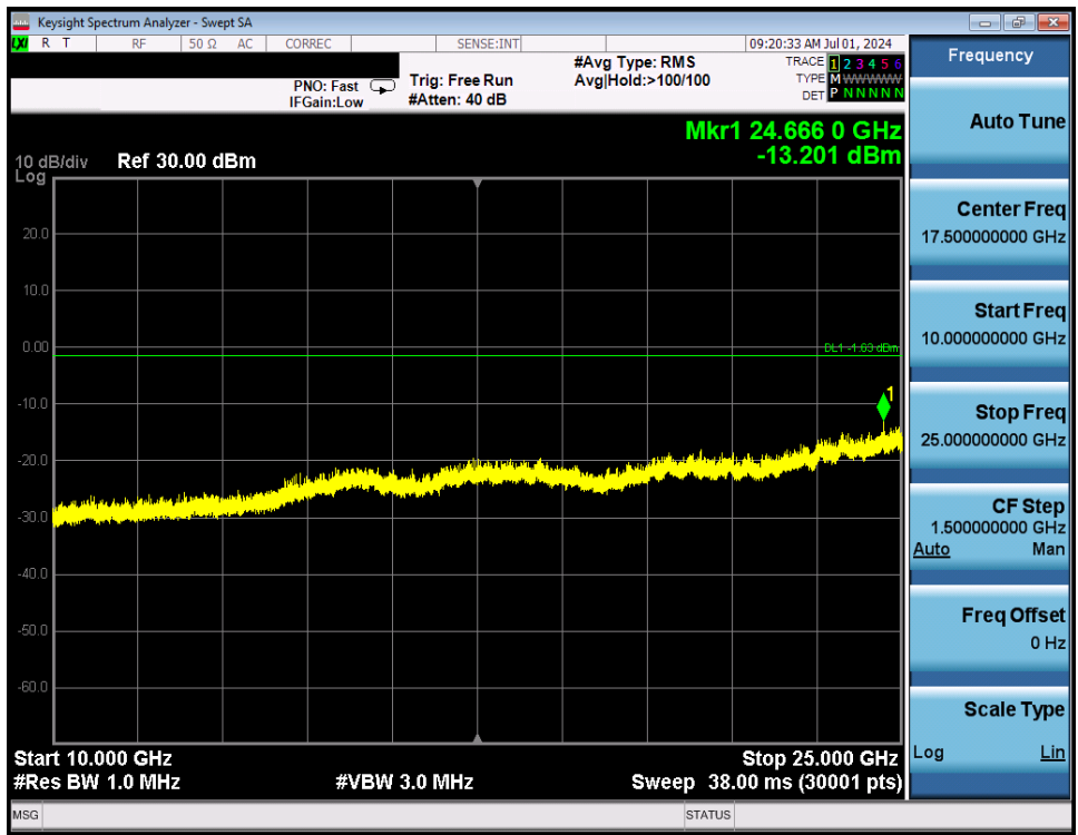
Plot 7-106. Conducted Spurious Plot Antenna WF8 (802.11ax OFDMA – RU26 – Ch. 1)
