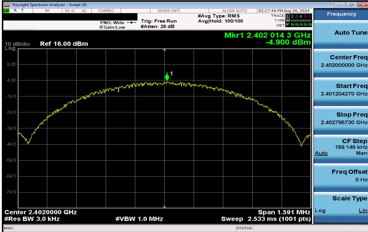
Plot 7-56. Power Spectral Density Plot Antenna WF7 (Bluetooth (LE), 1Mbps, iPA – Ch. 0)
