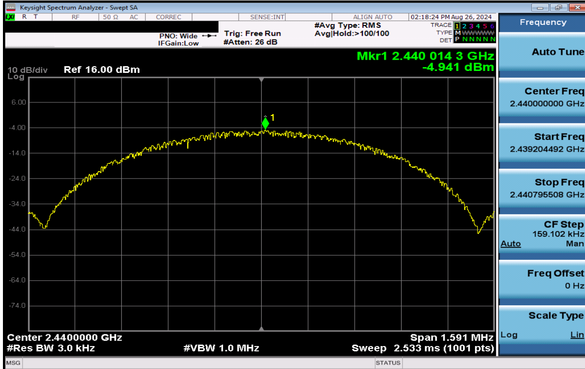
Plot 7-58. Power Spectral Density Plot Antenna WF7 (Bluetooth (LE), 1Mbps, iPA – Ch. 19)
