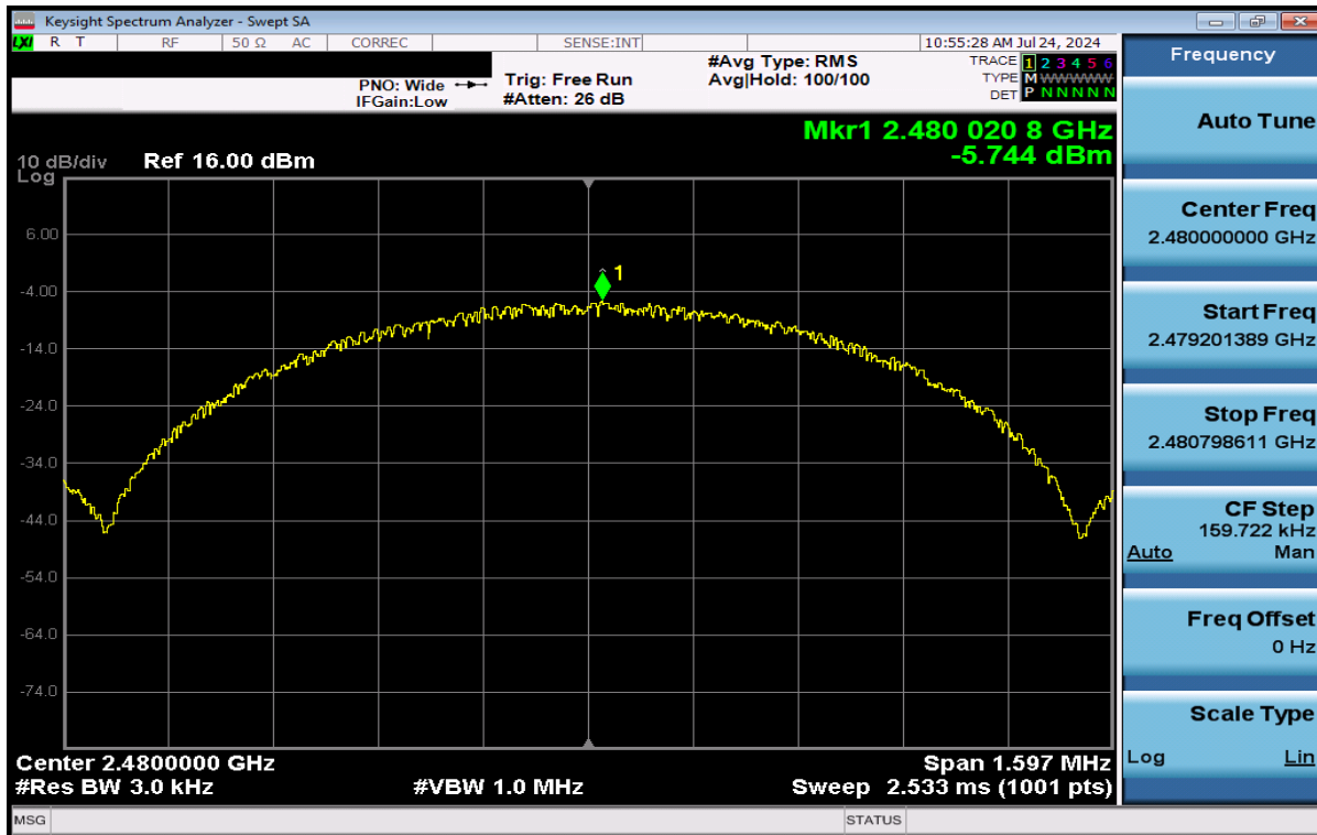
Plot 7-45. Power Spectral Density Plot Antenna WF2 (Bluetooth (LE), 1Mbps, iPA – Ch. 39)
