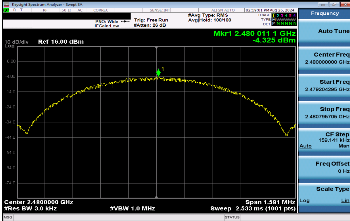
Plot 7-60. Power Spectral Density Plot Antenna WF7 (Bluetooth (LE), 1Mbps, iPA – Ch. 39)
