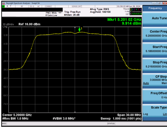
Plot 7-277. PSD Antenna WF2 (20MHz BW 802.11n – Ch. 40, MCS2)
