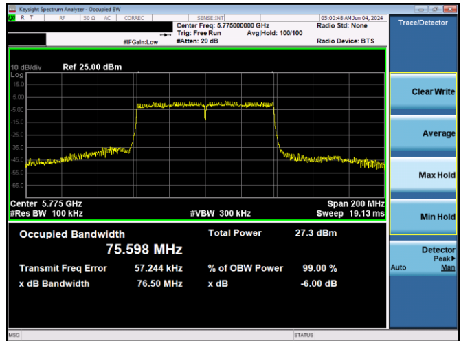
Plot 7-167. 6dB BW & 99% OBW Antenna WF2 (80MHz BW 802.11ac – Ch. 155, MCS9)
