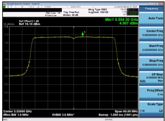
Plot 7-186. PSD Antenna WF5T (40MHz BW 802.11ax(SU) – Ch. 110, MCS2)
