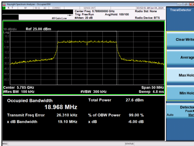
Plot 7-158. 6dB BW & 99% OBW Antenna WF2 (20MHz BW 802.11ax(SU) – Ch. 157, MCS4)
