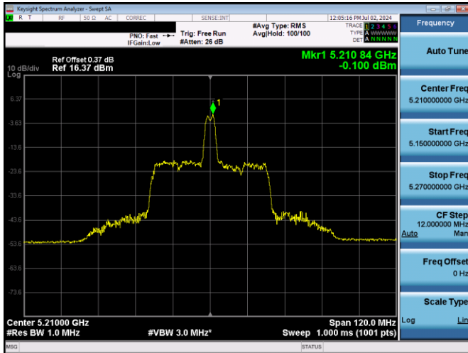
Plot 7-386. ISED PSD SDM Antenna WF2 (80MHz BW 11ax Index 18 - RU26 - Ch.42)
