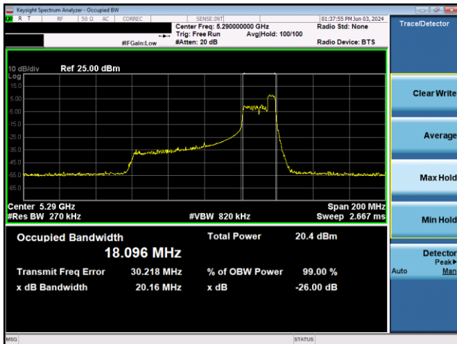
Plot 7-27. 26dB BW & 99% OBW Antenna WF5T (80MHz BW 11ax Index 52 – RU52 – Ch.58)
