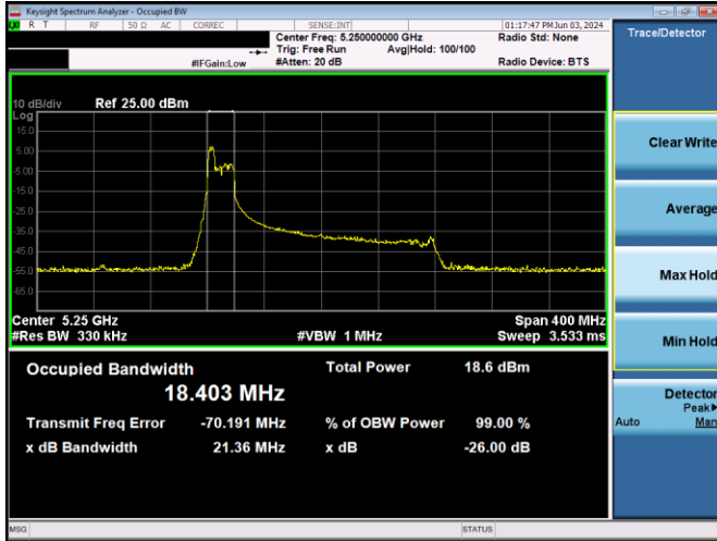
Plot 7-13. 26dB BW & 99% OBW Antenna WF5T (160MHz BW 11ax Index 37 - RU52 - Ch.50 (L))
