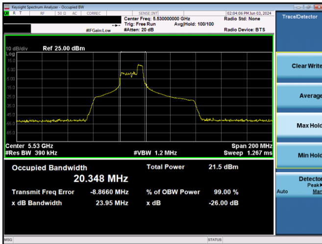
Plot 7-38. 26dB BW & 99% OBW Antenna WF5T (80MHz BW 11ax Index 44 – RU52 – Ch.106)
