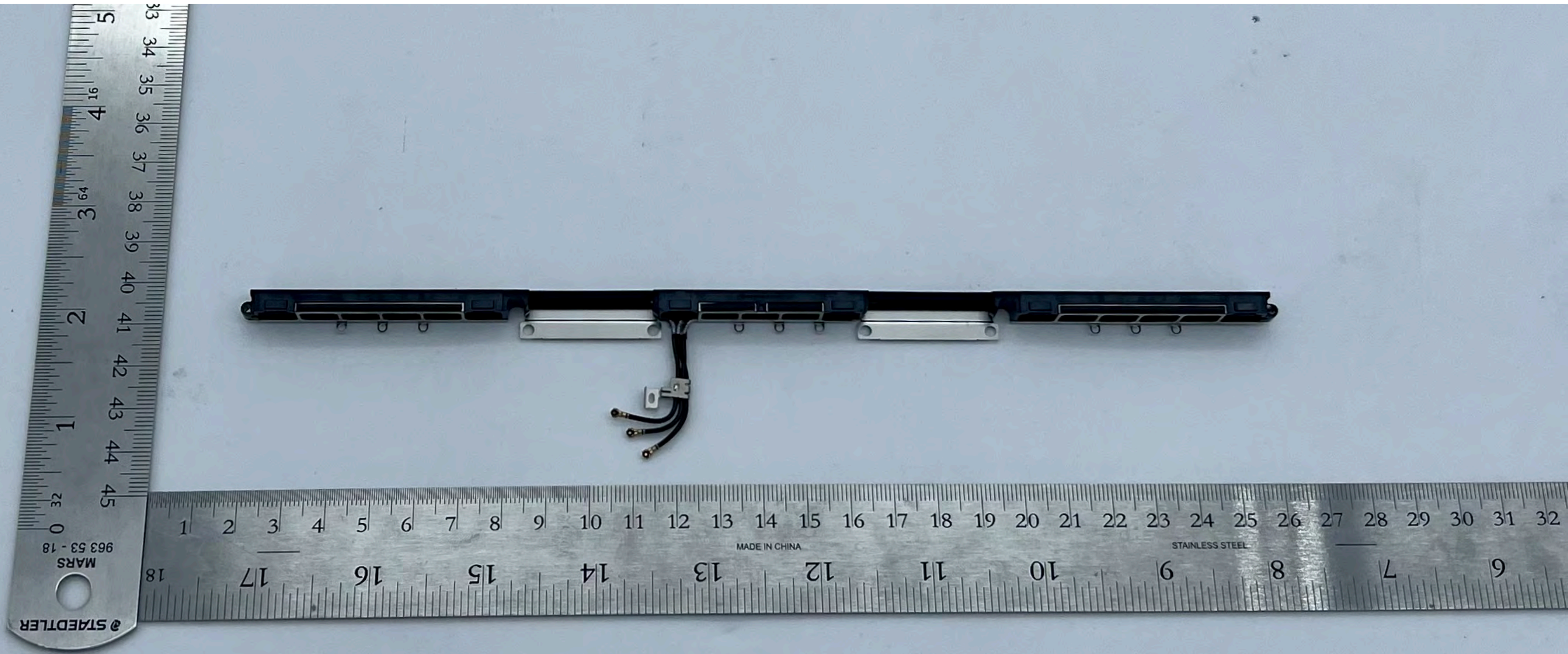
A2992 WF1/BT, WF2/BT, WF3 (BT) antenna structure and feed - Back
