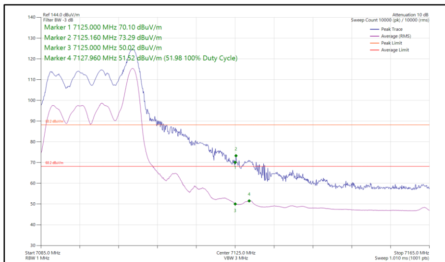
Figure 78 - 802.11ax HE20, RU 26-8, CDD, Core 0 + Core 1 - 7095 MHz Band Edge Frequency 7125 MHz
