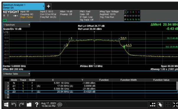
Figure 264 - 802.11n HT20 Minimum 99% OBW
