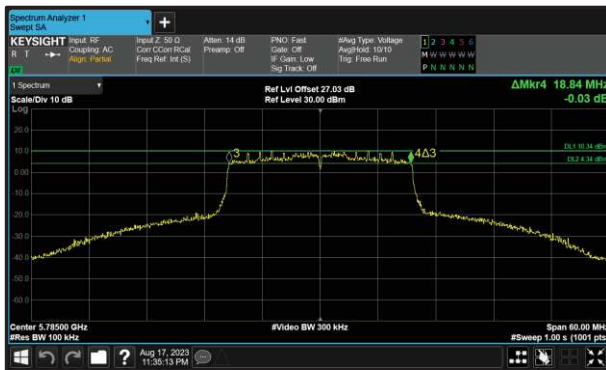
Figure 258 - 802.11ax HE20 SU Minimum 6 dB EBW
