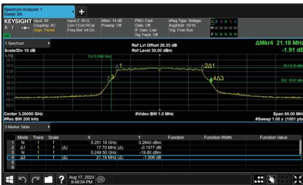
Figure 236 - 802.11n HT20 Minimum 99% OBW
