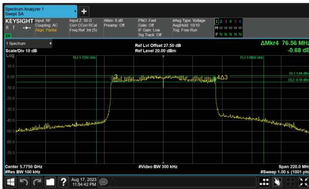
Figure 262 - 802.11ax HE80 SU Minimum 6 dB EBW
