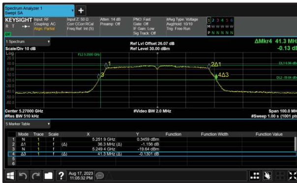
Figure 266 - 802.11n HT40 Minimum 99% OBW
