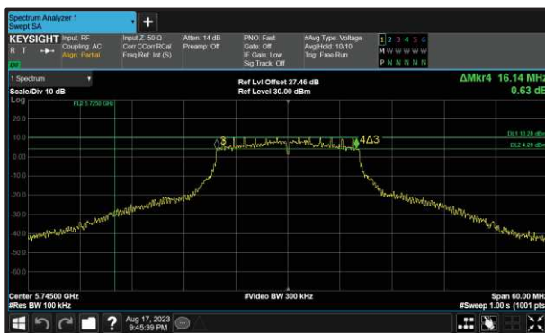
Figure 220 - 802.11a Minimum 6 dB EBW
