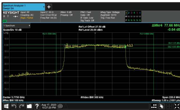
Figure 232 - 802.11ax HE80 SU Minimum 6 dB EBW
