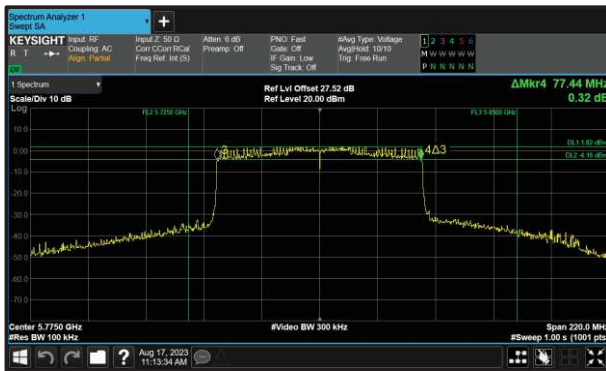
Figure 236 - 802.11ax HE80 SU Minimum 6 dB EBW
