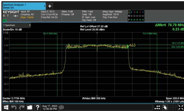
Figure 266 - 802.11ax HE80 SU Minimum 6 dB EBW
