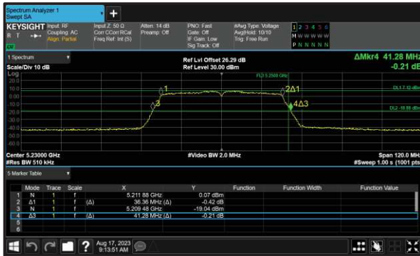
Figure 242 - 802.11n HT40 Minimum 99% OBW
