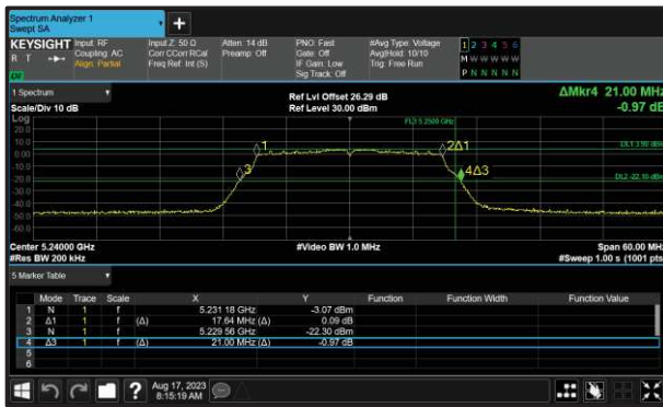
Figure 268 - 802.11n HT20 Minimum 99% OBW
