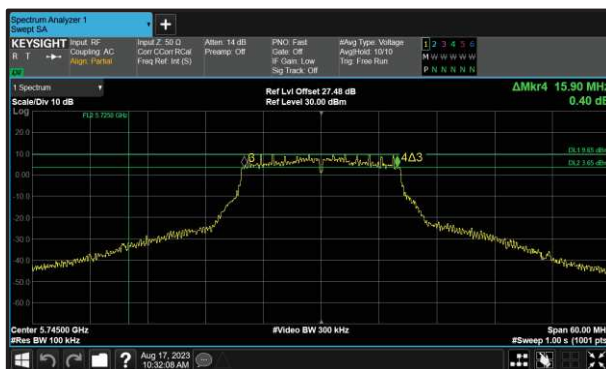
Figure 224 - 802.11a Minimum 6 dB EBW
