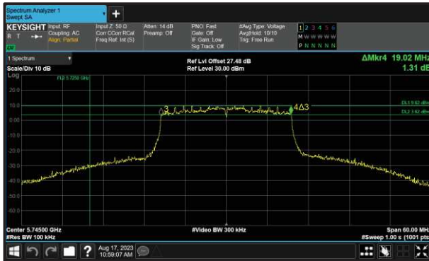
Figure 232 - 802.11ax HE20 SU Minimum 6 dB EBW
