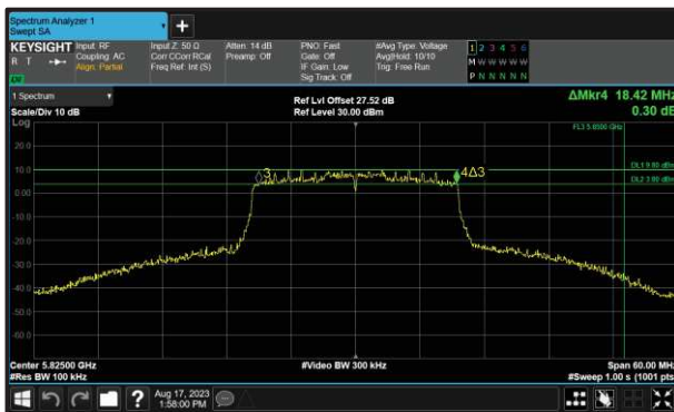
Figure 290 - 802.11ax HE20 SU Minimum 6 dB EBW
