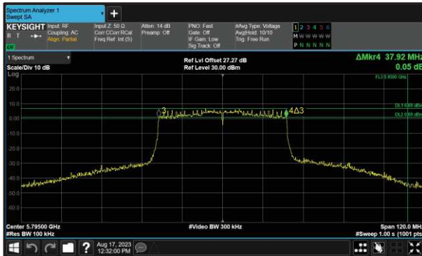
Figure 264 - 802.11ax HE40 SU Minimum 6 dB EBW
