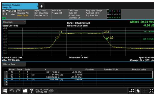
Figure 240 - 802.11n HT20 Minimum 99% OBW
