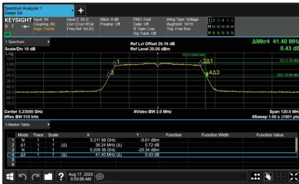
Figure 270 - 802.11n HT40 Minimum 99% OBW
