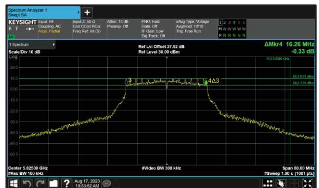
Figure 225 - 802.11a Maximum 6 dB EBW
