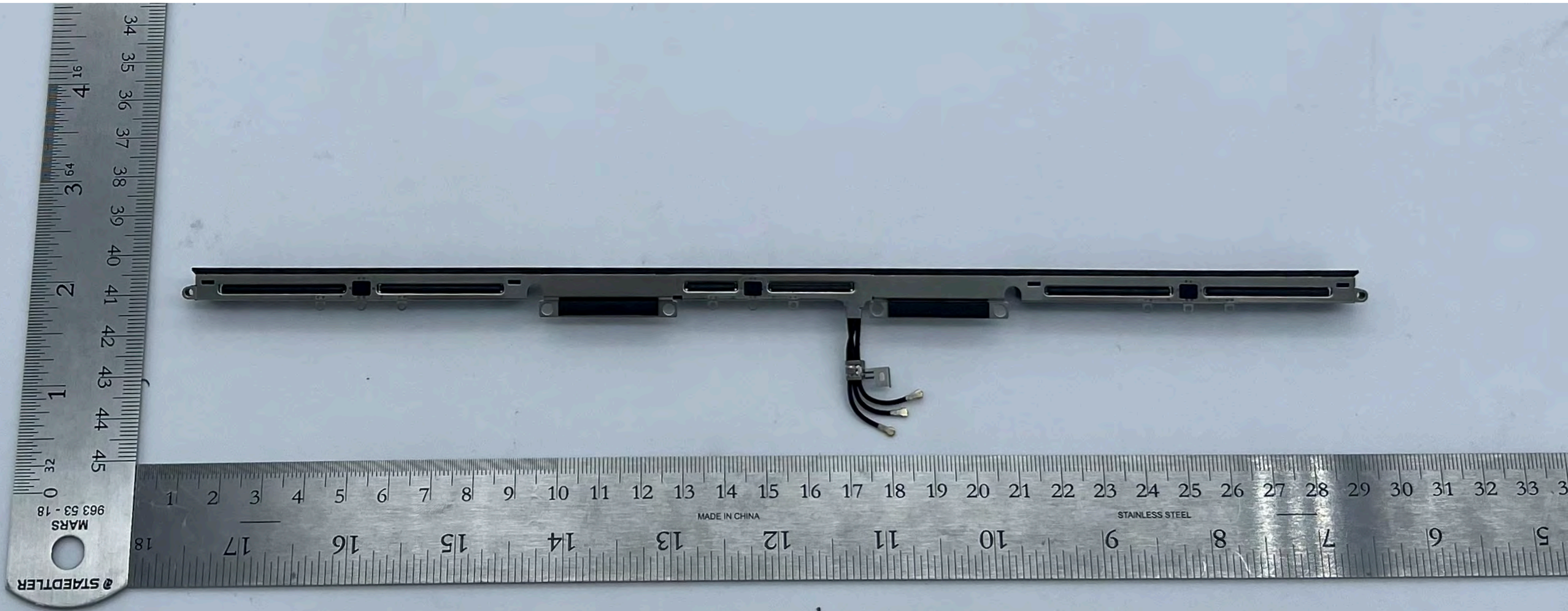
A2991 WF1/BT, WF2/BT, WF3 (BT) antenna structure and feed - Front
