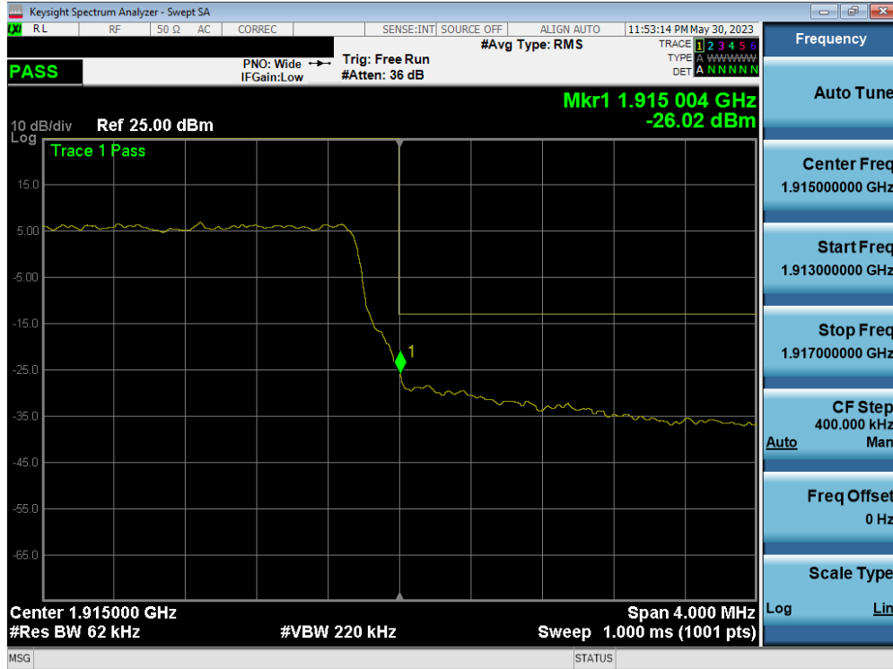
Plot 7-42. Upper Band Edge Plot (LTE Band 25 – 5MHz QPSK – Full RB Configuration)
