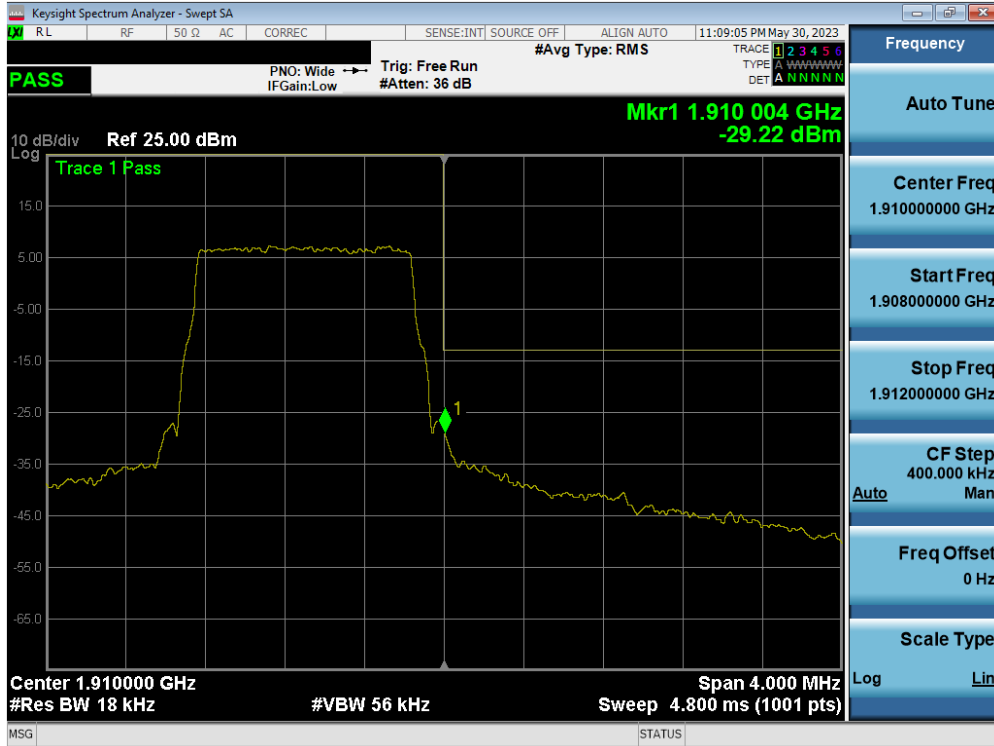
Plot 7-58. Upper Band Edge Plot (LTE Band 2 – 1.4MHz QPSK – Full RB Configuration)
