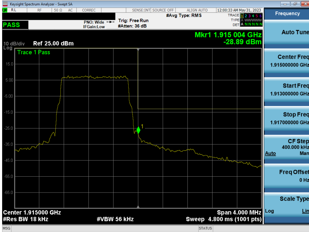
Plot 7-34. Upper Band Edge Plot (LTE Band 25 – 1.4MHz QPSK – Full RB Configuration)
