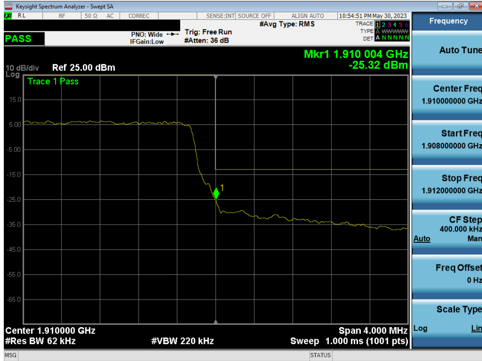
Plot 7-66. Upper Band Edge Plot (LTE Band 2 – 5MHz QPSK – Full RB Configuration)
