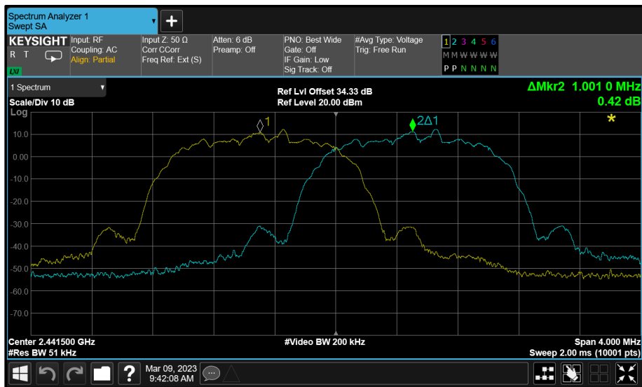
Figure 28 - 8-DPSK - 2441 MHz (CH39)
