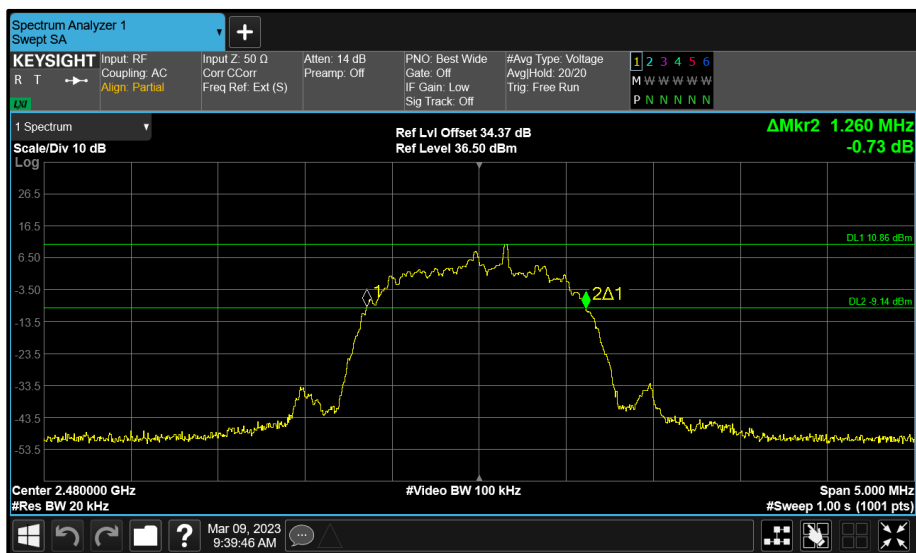
Figure 55 - Core 0 (B) 2480 MHz (CH78) 20 dB Bandwidth
