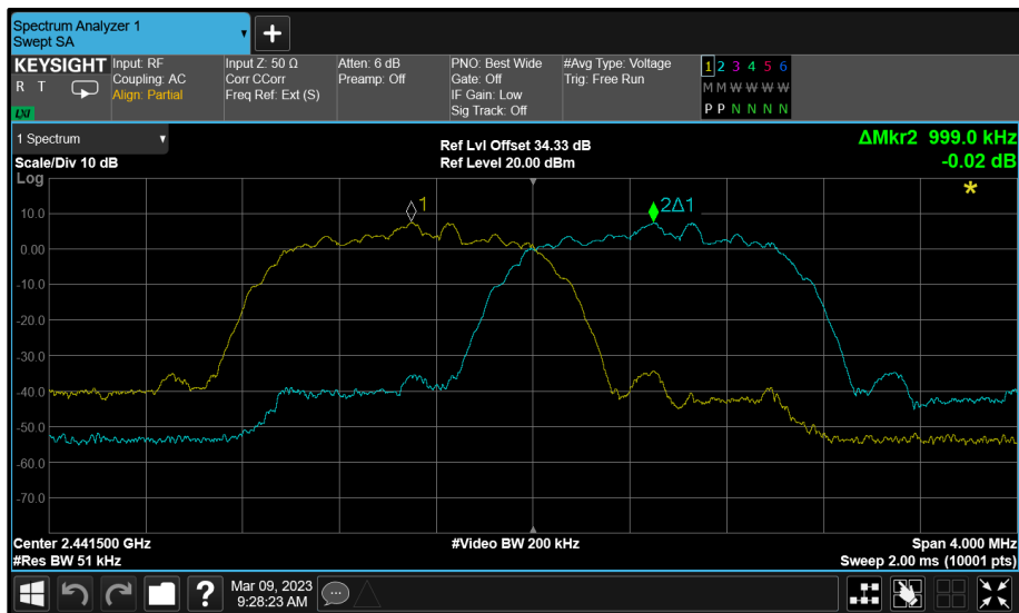
Figure 33 - \pi/4 DQPSK - 2441 MHz (CH39)
