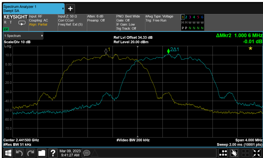
Figure 27 - \pi/4 DQPSK - 2441 MHz (CH39)
