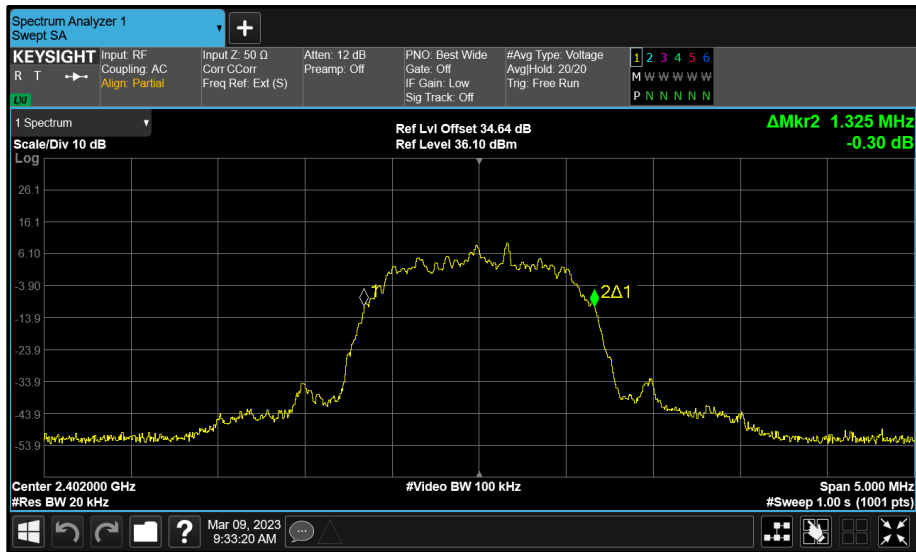
Figure 46 - Core 1 (C) 2402 MHz (CH0) 20 dB Bandwidth
