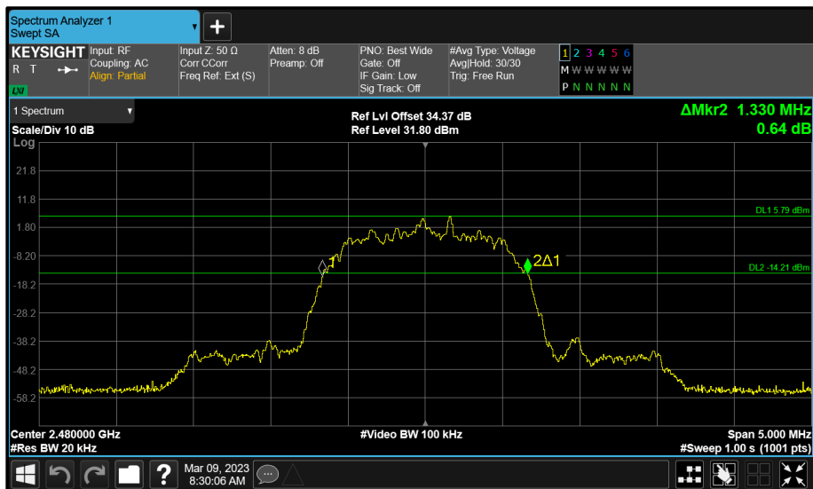
Figure 68 - Core 0 (B) 2480 MHz (CH78) 20 dB Bandwidth
