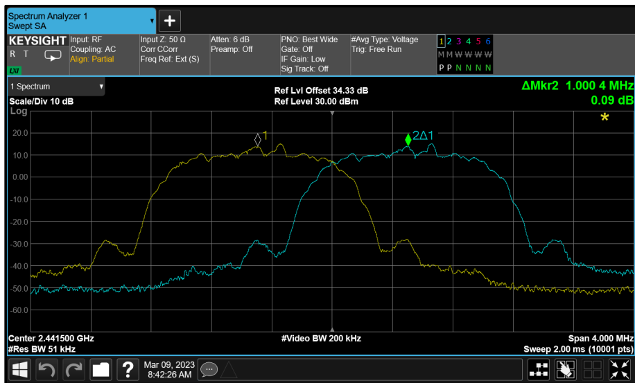
Figure 26 - 8-DPSK - 2441 MHz (CH39)
