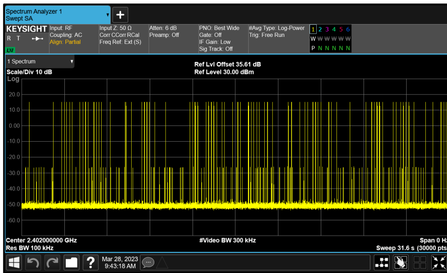
Figure 21 - \pi/4 DQPSK - 2402 MHz Accumulated Transmit Time
