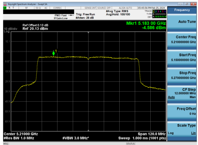
Plot 7-870. ISED PSD CDD Diversity Antenna 2a (80MHz BW 11ax(SU) - Ch.42, MCS2)
