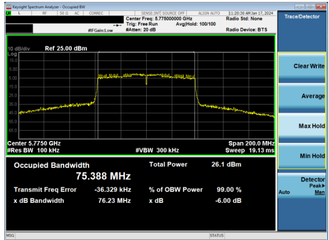
Plot 7-245. 6dB BW & 99% OBW Antenna 2a (80MHz BW 802.11ac – Ch. 155, MCS4)
