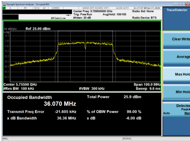
Plot 7-243. 6dB BW & 99% OBW Antenna 2a (40MHz BW 802.11n – Ch. 151, MCS4)
