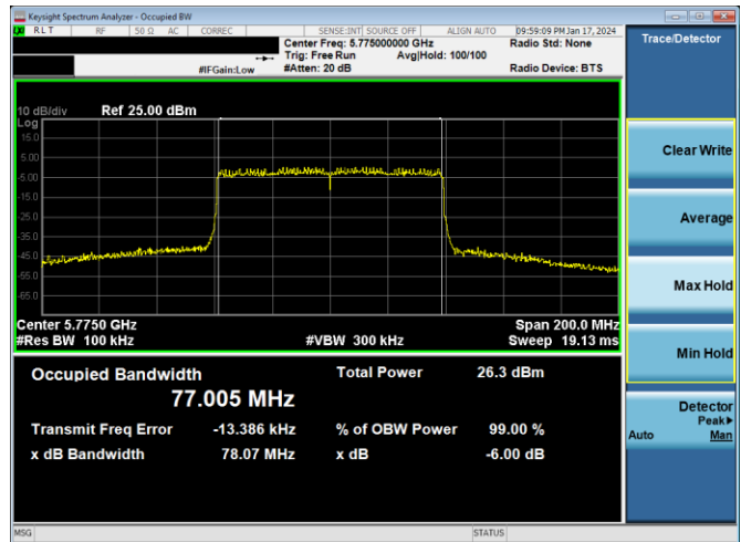
Plot 7-234. 6dB BW & 99% OBW Antenna 4a (80MHz BW 802.11ax(SU) – Ch. 155, MCS11)
