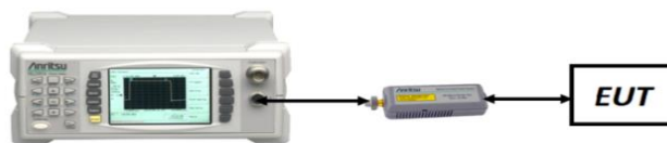
Figure 7-3. Test Instrument & Measurement Setup
