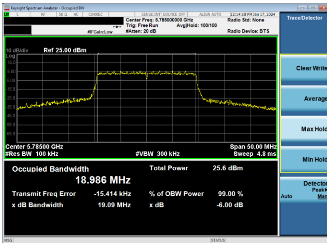
Plot 7-248. 6dB BW & 99% OBW Antenna 2a (20MHz BW 802.11ax(SU) – Ch. 157, MCS11)
