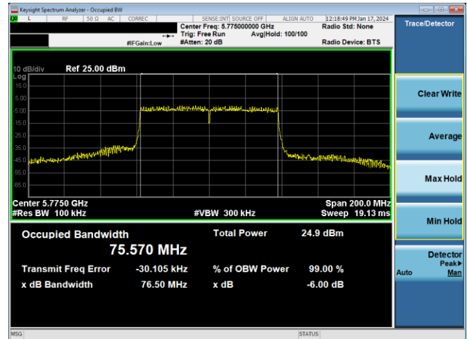
Plot 7-251. 6dB BW & 99% OBW Antenna 2a (80MHz BW 802.11ac – Ch. 155, MCS9)
