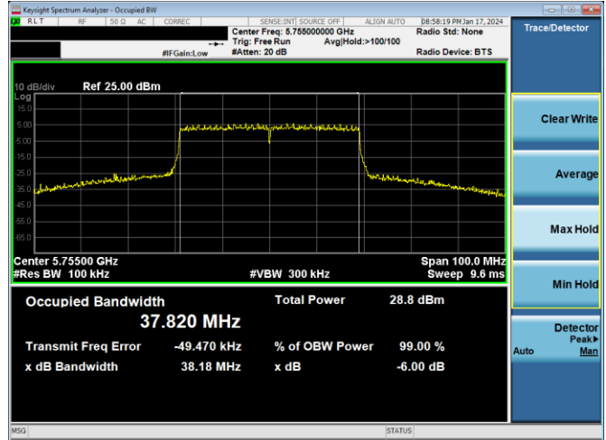
Plot 7-226. 6dB BW & 99% OBW Antenna 4a (40MHz BW 802.11ax(SU) – Ch. 151, MCS4)
