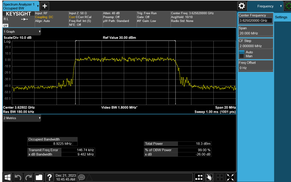
Plot 7-37. Occupied Bandwidth Plot (NR Band n48 - 10MHz CP-OFDM 256-QAM - Full RB Configuration)
