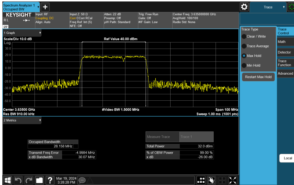
Plot 7-21. Occupied Bandwidth Plot (ULCA LTE Band 48 - 20+10MHz QPSK - Full RB Configuration)
