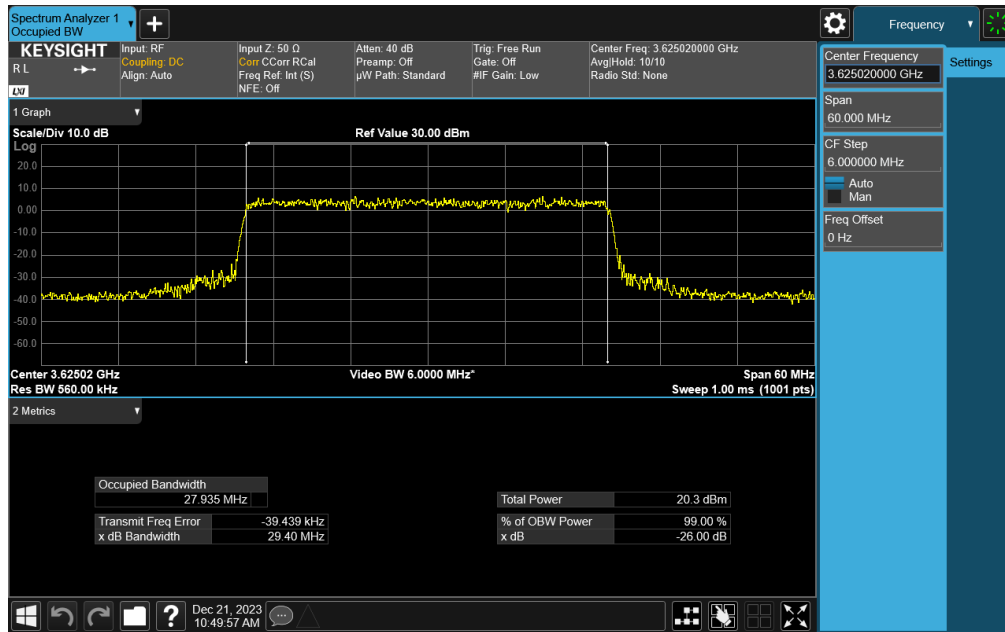
Plot 7-51. Occupied Bandwidth Plot (NR Band n48 - 30MHz CP-OFDM 64-QAM - Full RB Configuration)
