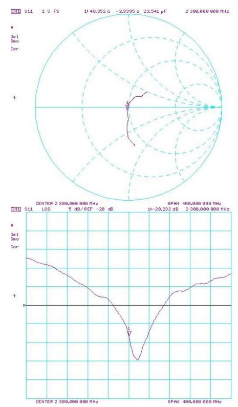
Impedance & Return-Loss Measurement Plot for Head TSL
