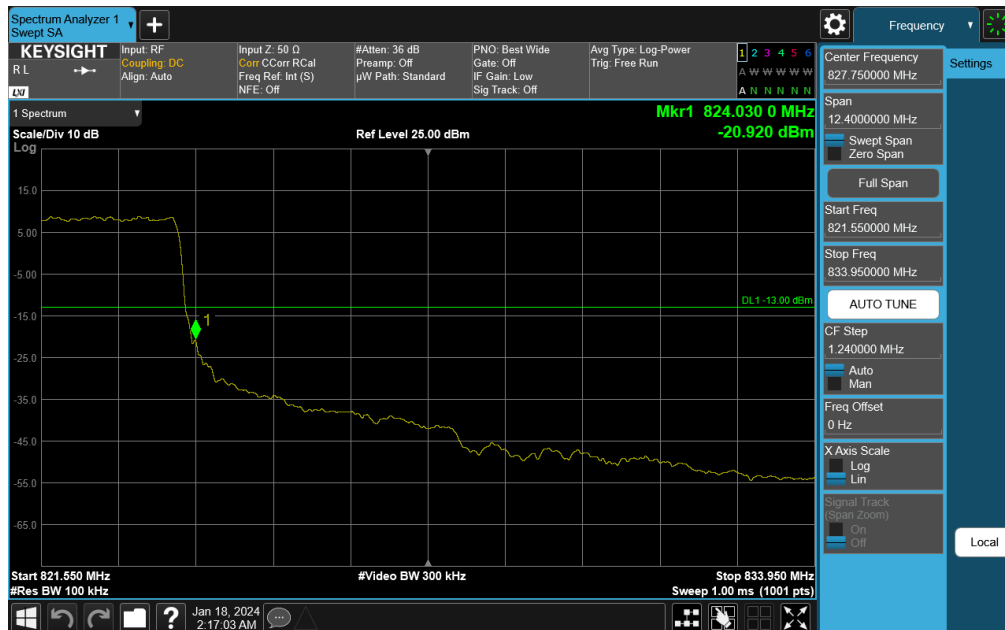
Plot 7-115. Upper Band Edge Plot (NR Band n26 - 5MHz DFT-s-OFDM QPSK – High Channel)
