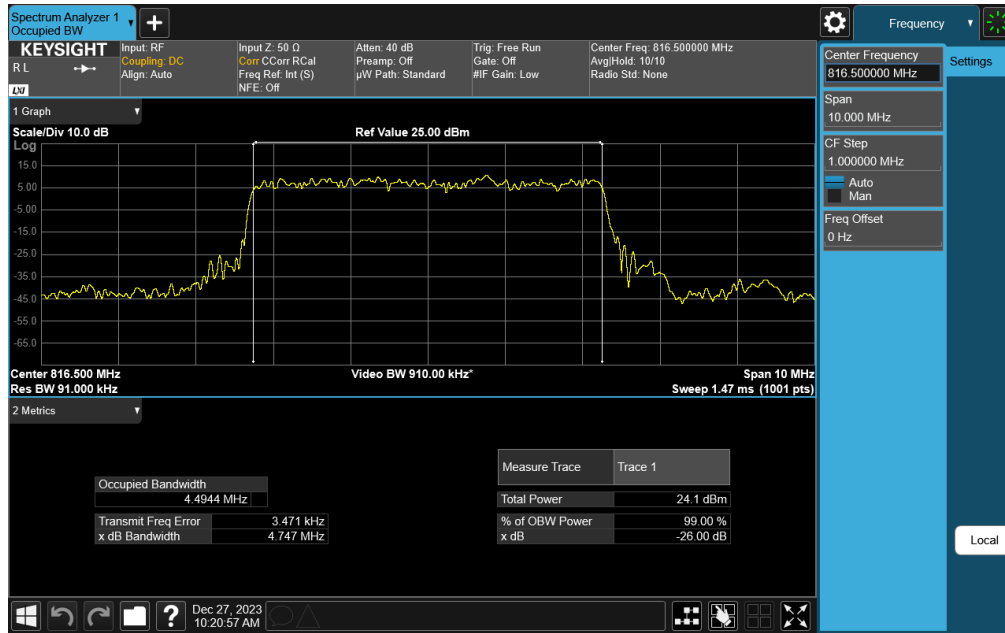
Plot 7-35. Occupied Bandwidth Plot (NR Band 26 - 5MHz DFT-s-OFDM \pi/2 BPSK - Full RB)
