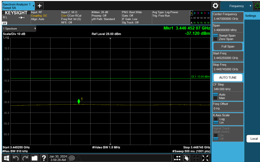
Plot 7-210. Lower ACP Plot (NR Band n77 DoD-Band - 100MHz DFT-s-OFDM QPSK – Full RB)
