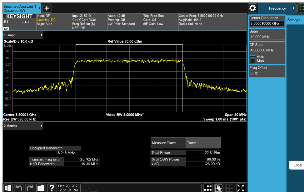
Plot 7-14. Occupied Bandwidth Plot (NR Band n77 DoD-Band - 20MHz CP-OFDM 64-QAM - Full RB)
