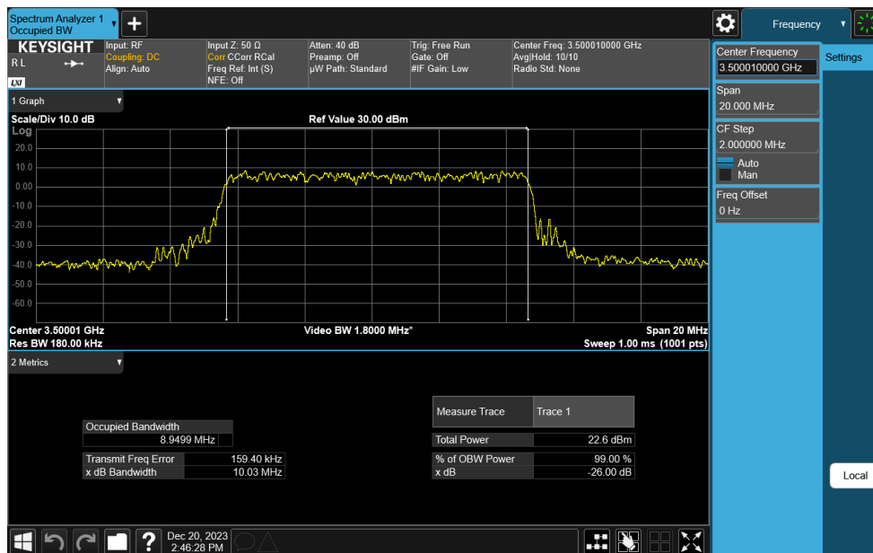
Plot 7-4. Occupied Bandwidth Plot (NR Band n77 DoD-Band - 10MHz CP-OFDM 64-QAM - Full RB)
