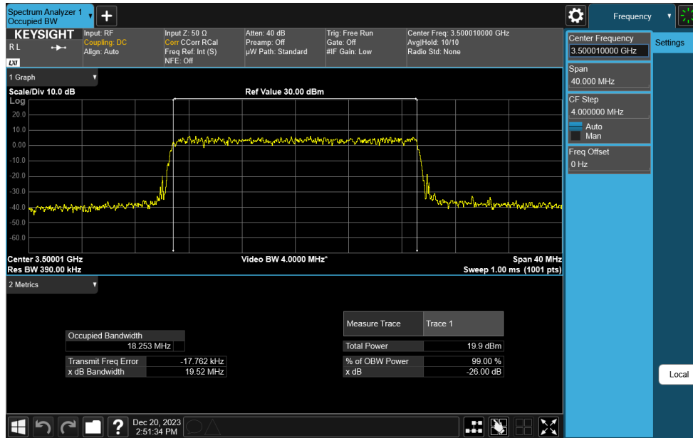
Plot 7-15. Occupied Bandwidth Plot (NR Band n77 DoD-Band - 20MHz CP-OFDM 256-QAM - Full RB)
