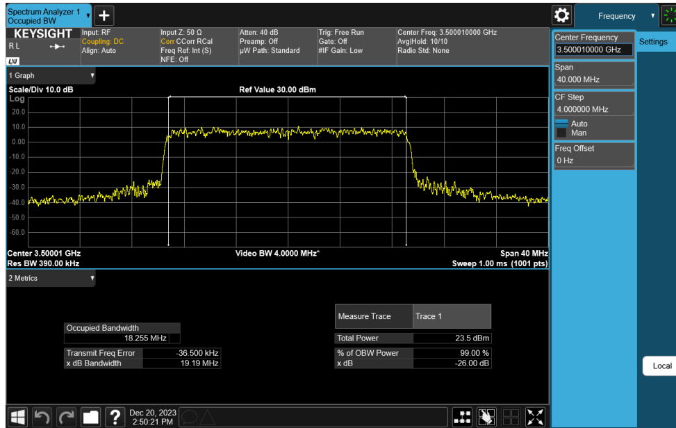
Plot 7-13. Occupied Bandwidth Plot (NR Band n77 DoD-Band - 20MHz CP-OFDM 16-QAM - Full RB)
