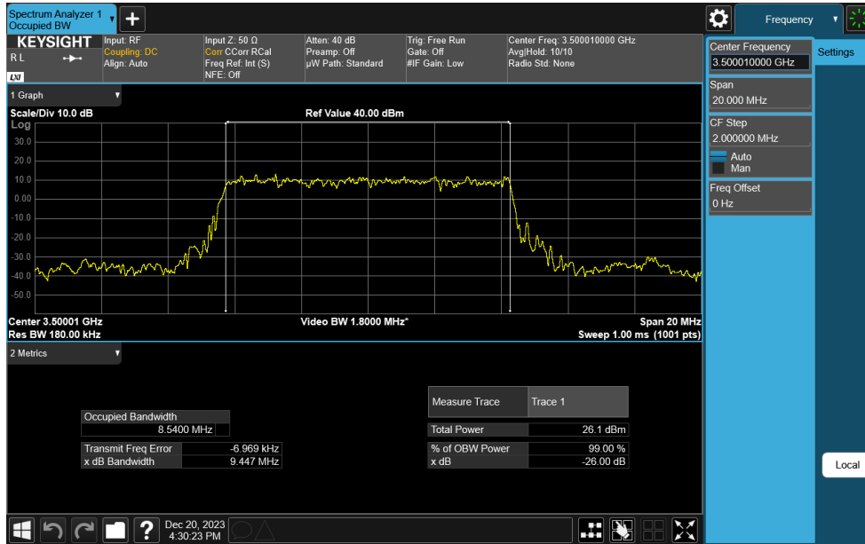
Plot 7-1. Occupied Bandwidth Plot (NR Band n77 DoD-Band - 10MHz DFT-s-OFDM \pi/2 BPSK - Full RB)
