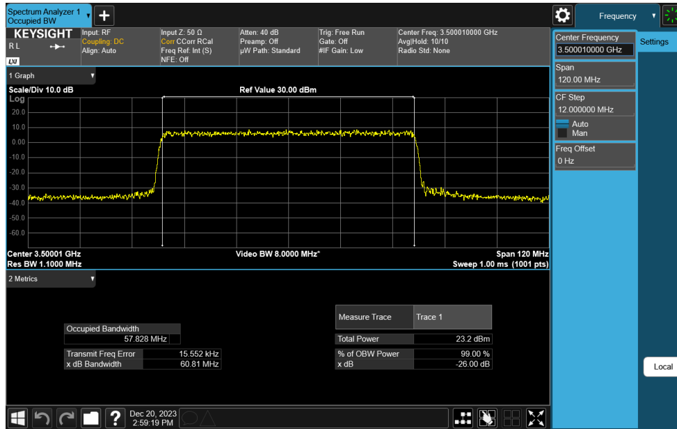
Plot 7-33. Occupied Bandwidth Plot (NR Band n77 DoD-Band - 60MHz CP-OFDM 16-QAM - Full RB)
