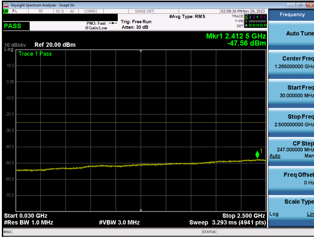
Plot 7-214. Conducted Spurious Plot (ULCA LTE Band 7 – (20+20)MHz QPSK – RB Size 1, RB Offset 0 – High Channel)
