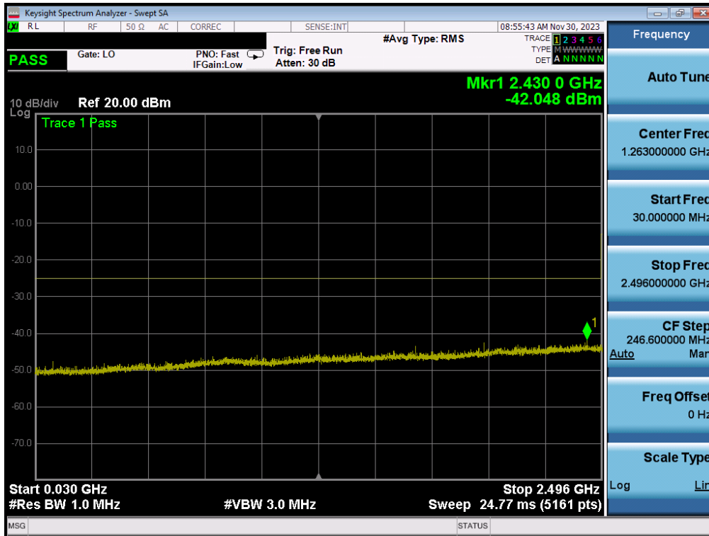
Plot 7-223. Conducted Spurious Plot (ULCA LTE Band 41 – (20+20)MHz QPSK – RB Size 1, RB Offset 0 – High Channel)
