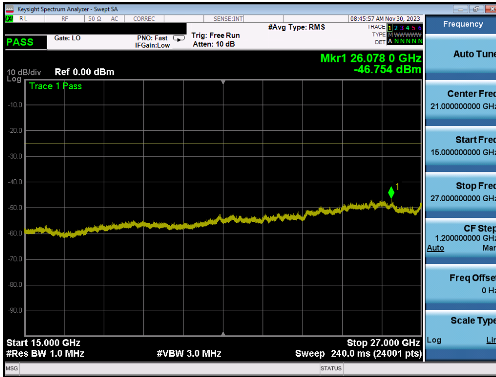
Plot 7-219. Conducted Spurious Plot (ULCA LTE Band 41 – (20+20)MHz QPSK – RB Size 1, RB Offset 0 – Low Channel)
