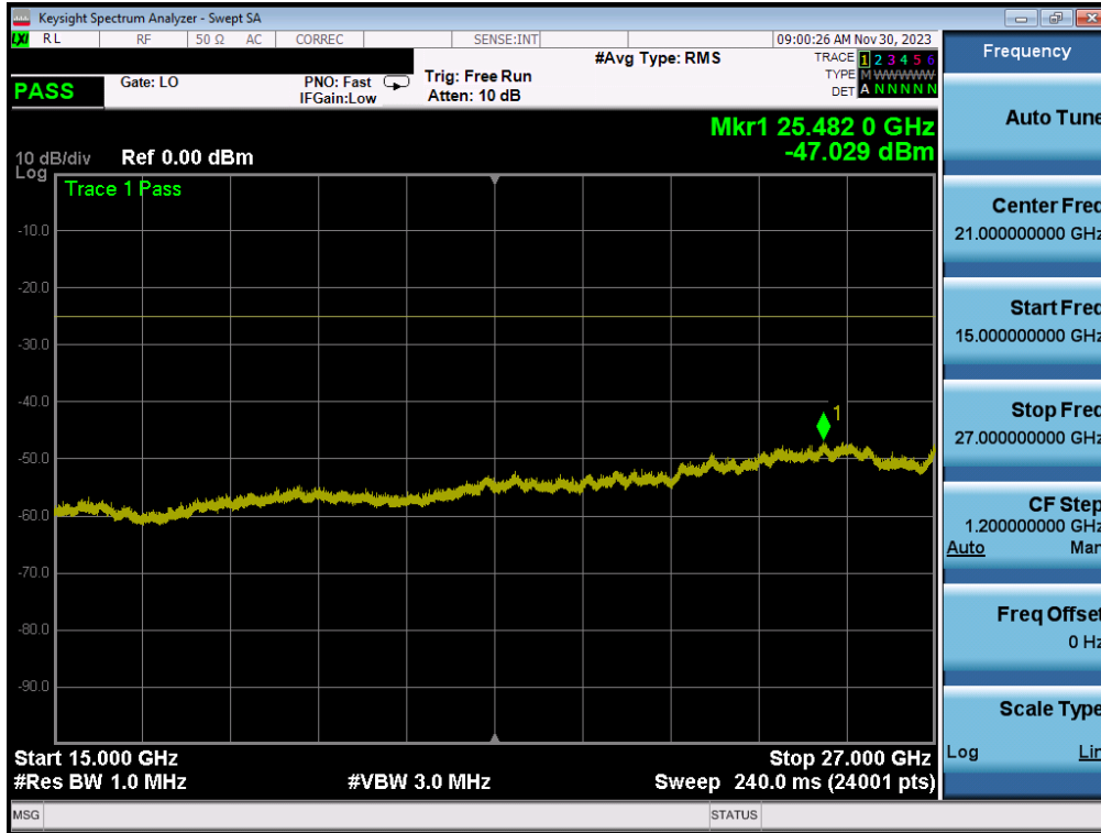
Plot 7-225. Conducted Spurious Plot (ULCA LTE Band 41 – (20+20)MHz QPSK – RB Size 1, RB Offset 0 – High Channel)
