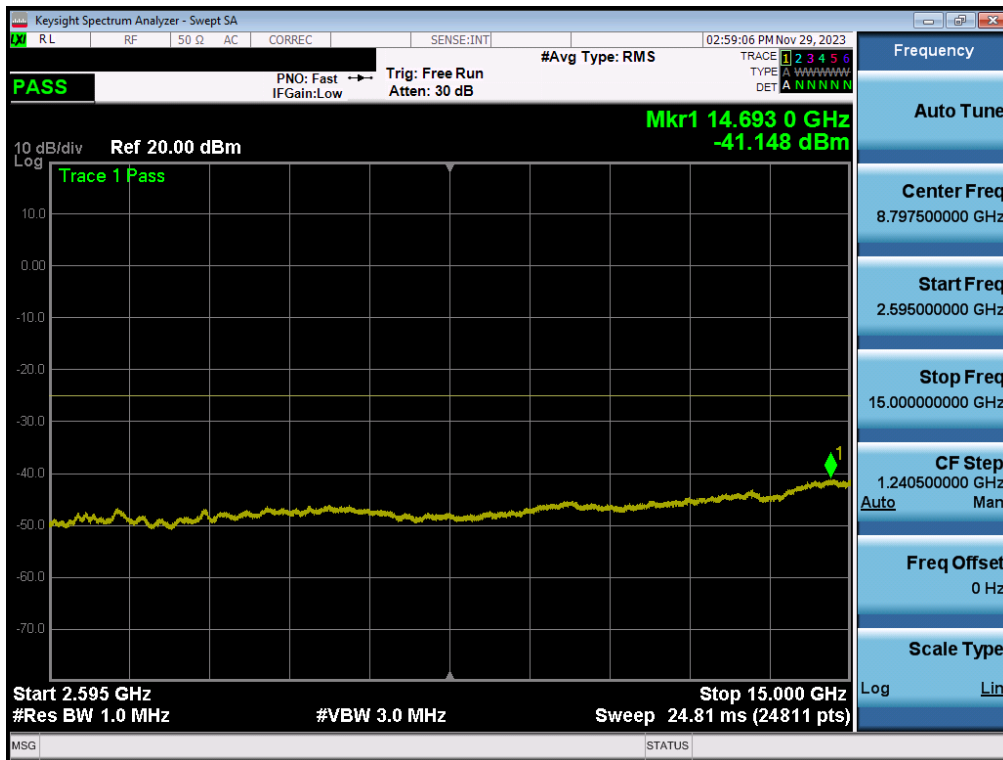
Plot 7-215. Conducted Spurious Plot (ULCA LTE Band 7 – (20+20)MHz QPSK – RB Size 1, RB Offset 0 – High Channel)
