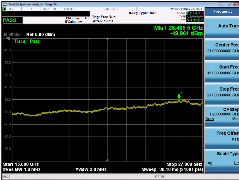
Plot 7-216. Conducted Spurious Plot (ULCA LTE Band 7 – (20+20)MHz QPSK – RB Size 1, RB Offset 0 – High Channel)
