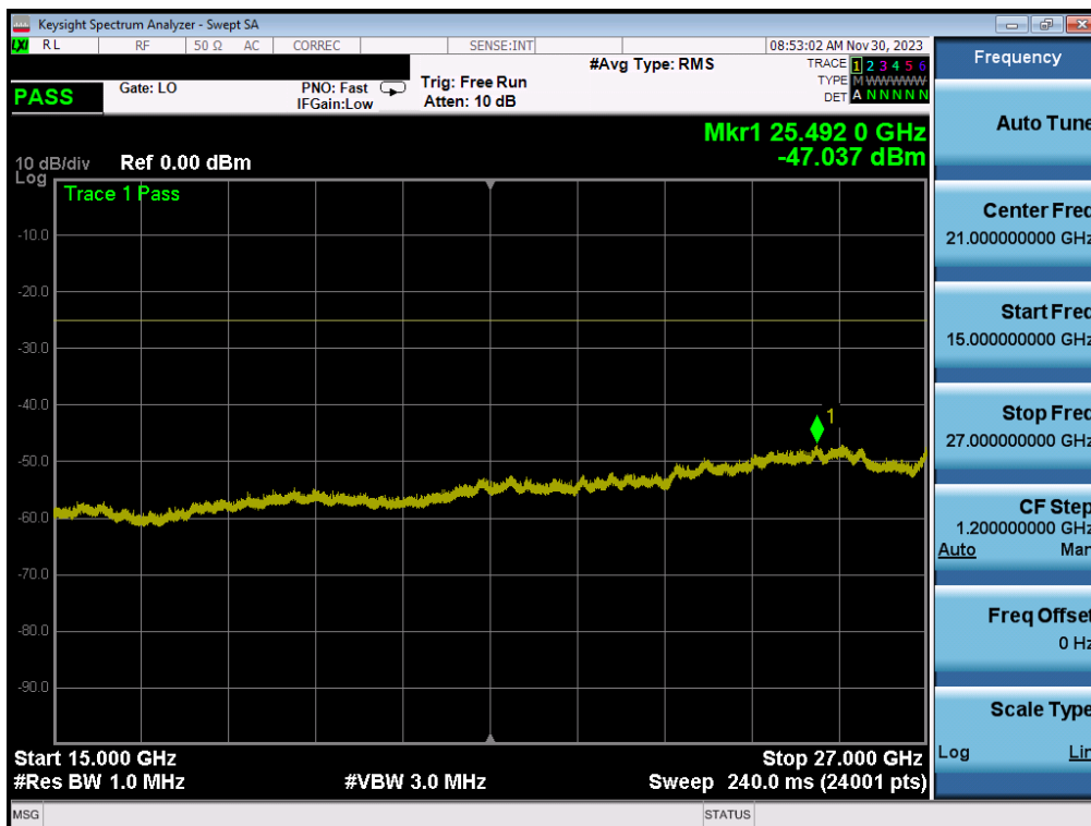
Plot 7-222. Conducted Spurious Plot (ULCA LTE Band 41 – (20+20)MHz QPSK – RB Size 1, RB Offset 0 – Mid Channel)
