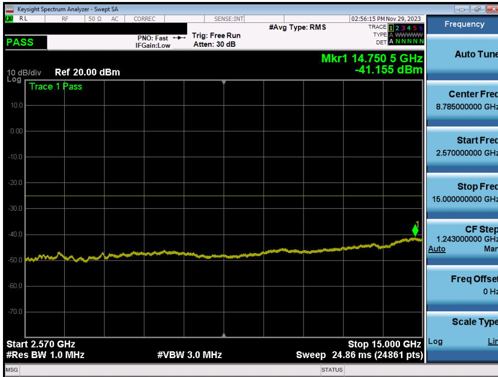
Plot 7-212. Conducted Spurious Plot (ULCA LTE Band 7 – (20+20)MHz QPSK – RB Size 1, RB Offset 0 – Mid Channel)
