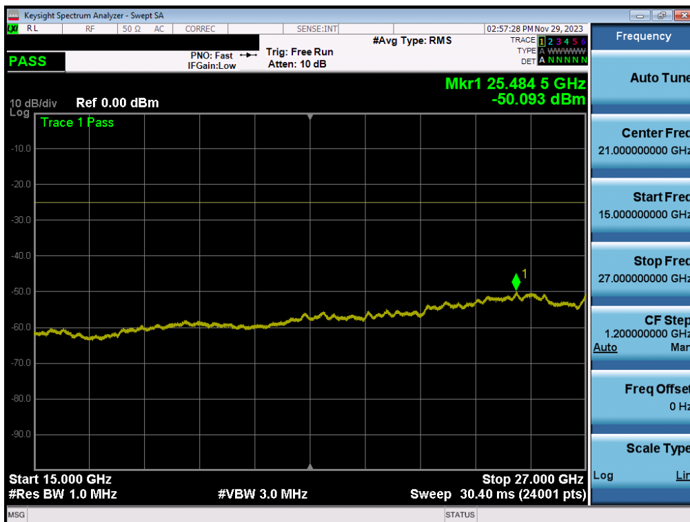
Plot 7-213. Conducted Spurious Plot (ULCA LTE Band 7 – (20+20)MHz QPSK – RB Size 1, RB Offset 0 – Mid Channel)
