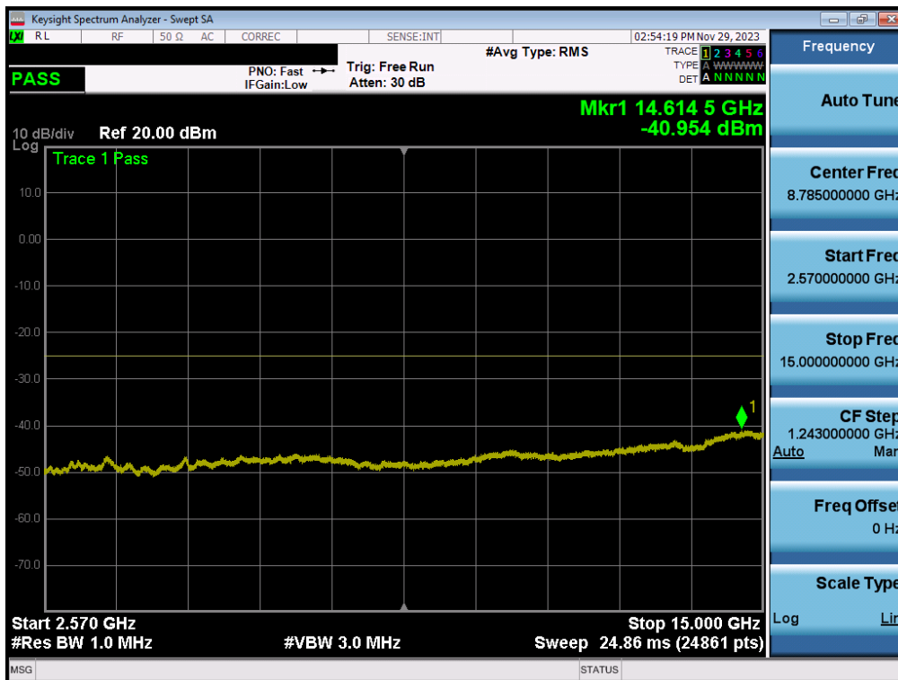
Plot 7-209. Conducted Spurious Plot (ULCA LTE Band 7 – (20+20)MHz QPSK – RB Size 1, RB Offset 0 – Low Channel)
