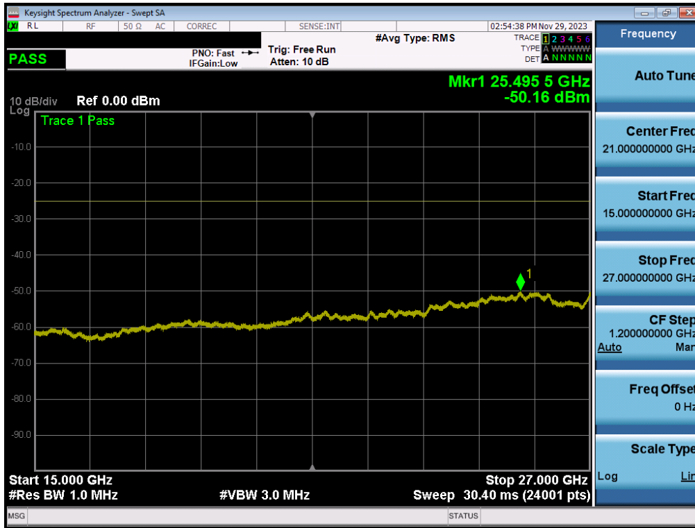
Plot 7-210. Conducted Spurious Plot (ULCA LTE Band 7 – (20+20)MHz QPSK – RB Size 1, RB Offset 0 – Low Channel)
