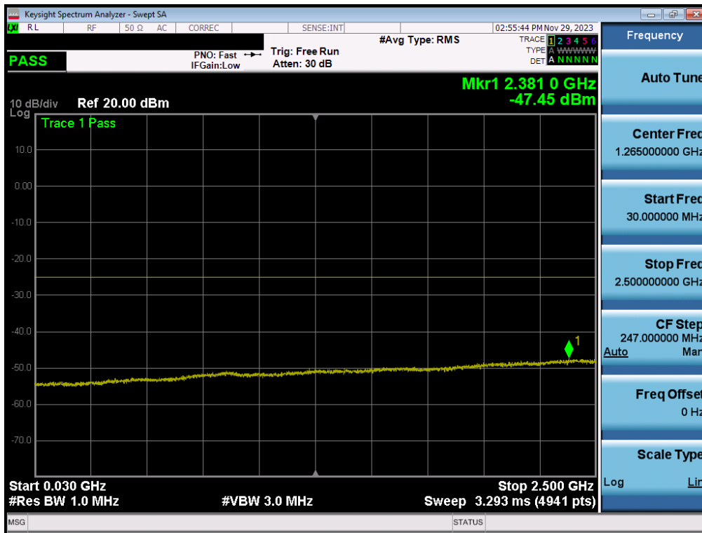
Plot 7-211. Conducted Spurious Plot (ULCA LTE Band 7 – (20+20)MHz QPSK – RB Size 1, RB Offset 0 – Mid Channel)
