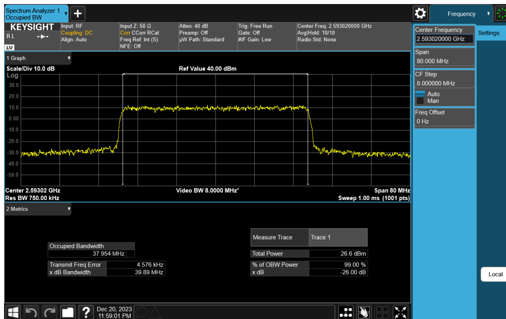
Plot 7-112. Occupied Bandwidth Plot (NR Band n41 - 40MHz CP-OFDM QPSK - Full RB)
