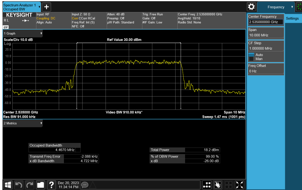
Plot 7-55. Occupied Bandwidth Plot (NR Band n7 - 5MHz DFT-s-OFDM 256-QAM - Full RB)
