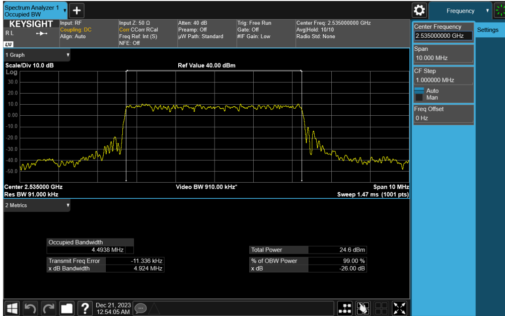
Plot 7-51. Occupied Bandwidth Plot (NR Band n7 - 5MHz DFT-s-OFDM \pi/2 BPSK - Full RB)
