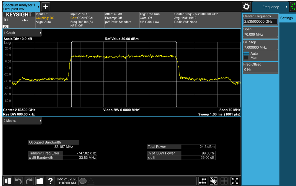
Plot 7-81. Occupied Bandwidth Plot (NR Band n7 - 35MHz DFT-s-OFDM \pi/2 BPSK - Full RB)
