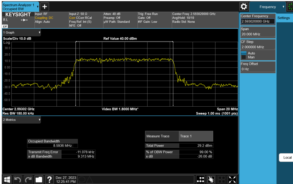
Plot 7-91. Occupied Bandwidth Plot (NR Band n41 - 10MHz DFT-s-OFDM \pi/2 BPSK - Full RB)
