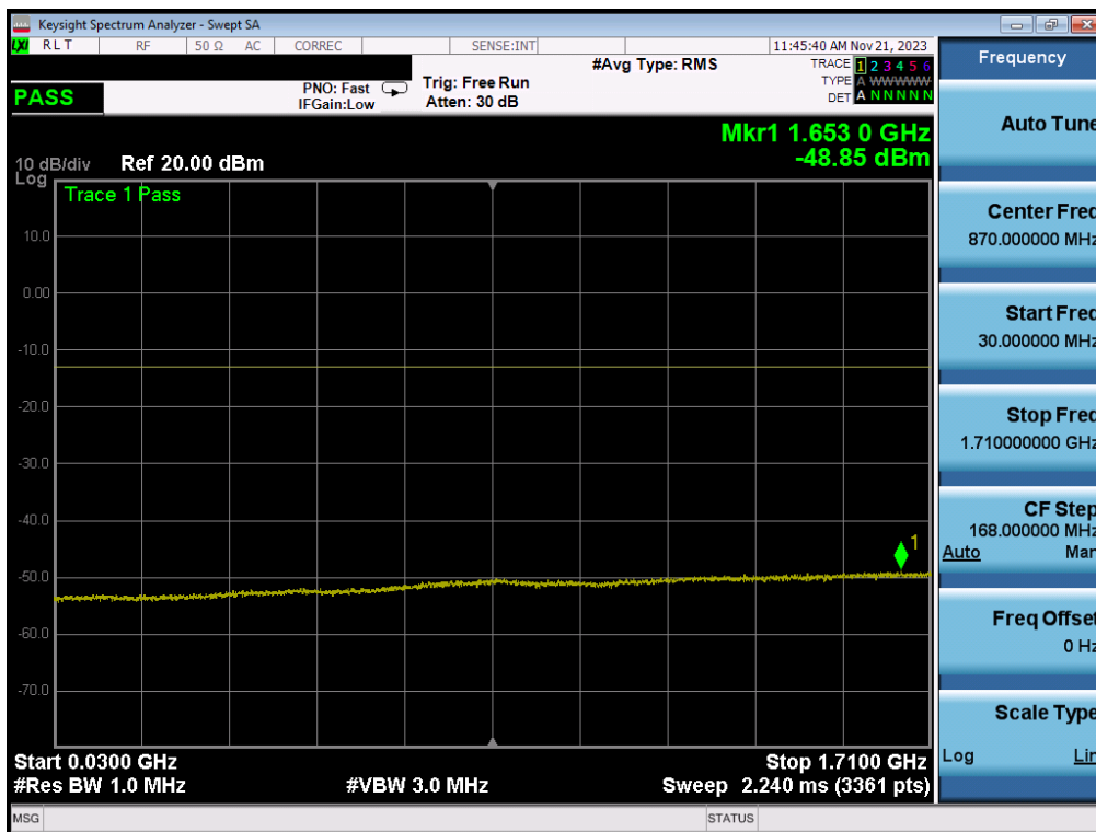
Plot 7-230. Conducted Spurious Plot (WCDMA Ch. 1413- Mid Channel)
