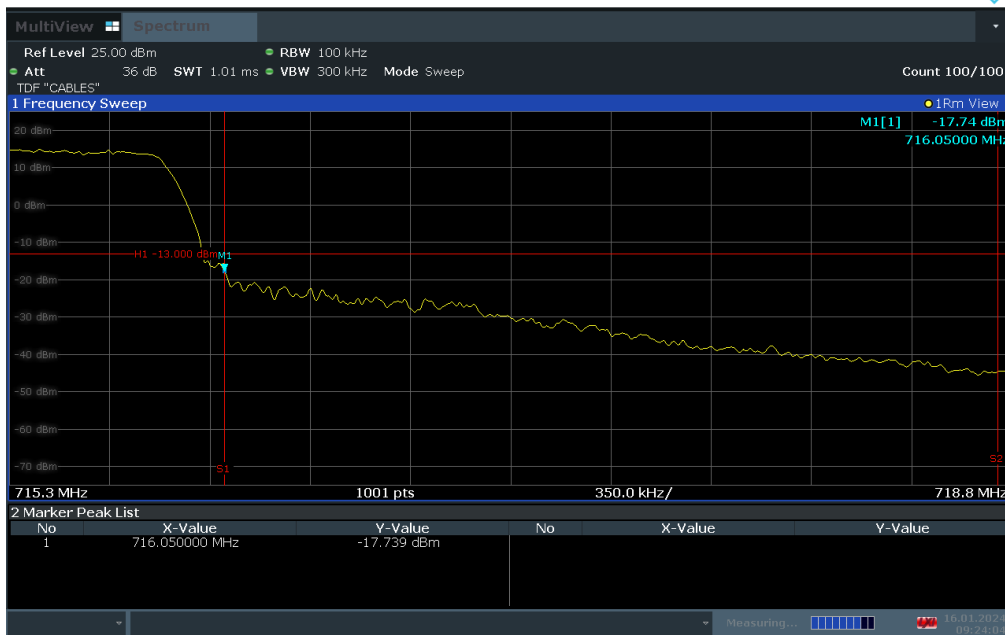
Plot 7-293. Upper Band Edge Plot (LTE Band 12 – 1.4MHz QPSK – Full RB)
