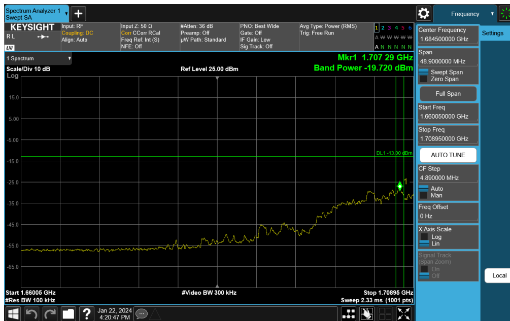
Plot 7-321. Lower Extended Band Edge Plot (NR Band n66 – 15.0MHz DFT-s-OFDM \pi/2 BPSK - Full RB)
