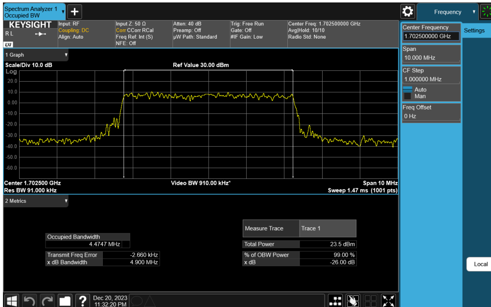
Plot 7-106. Occupied Bandwidth Plot (NR Band n70 - 5MHz CP-OFDM QPSK - Full RB)
