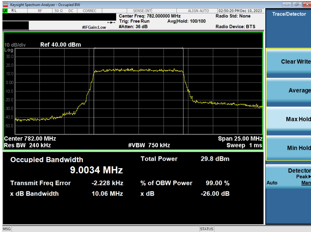
Plot 7-64. Occupied Bandwidth Plot (LTE Band 13 - 10MHz 256-QAM - Full RB)
