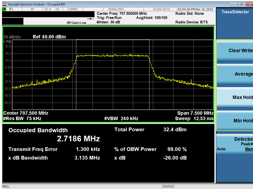
Plot 7-46. Occupied Bandwidth Plot (LTE Band 12 - 3MHz 16-QAM - Full RB)
