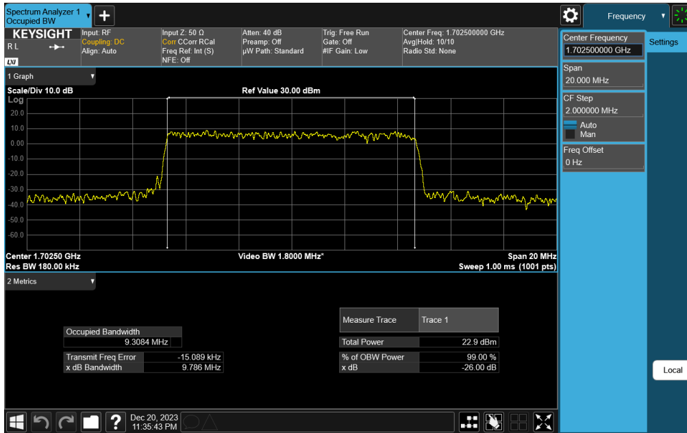
Plot 7-113. Occupied Bandwidth Plot (NR Band n70 - 10MHz CP-OFDM 64-QAM - Full RB)
