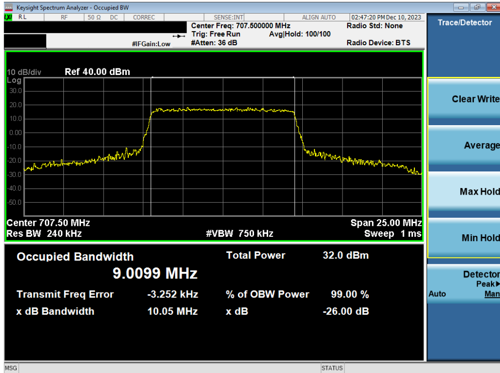
Plot 7-55. Occupied Bandwidth Plot (LTE Band 12/17 - 10MHz 64-QAM - Full RB)
