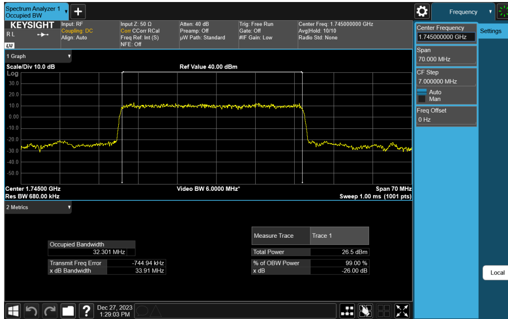
Plot 7-95. Occupied Bandwidth Plot (NR Band n66 - 35.0MHz DFT-s-OFDM \pi/2 BPSK - Full RB)
