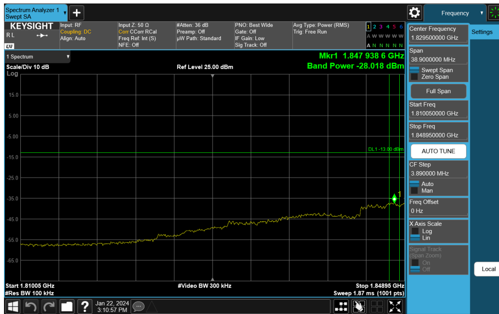
Plot 7-170. Extended Lower Band Edge Plot (NR Band n25 – 40MHz DFT-s-OFDM \pi/2 BPSK – Full RB Configuration)
