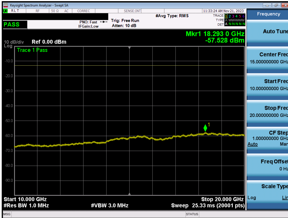
Plot 7-89. Conducted Spurious Plot (WCDMA Ch. 9400)
