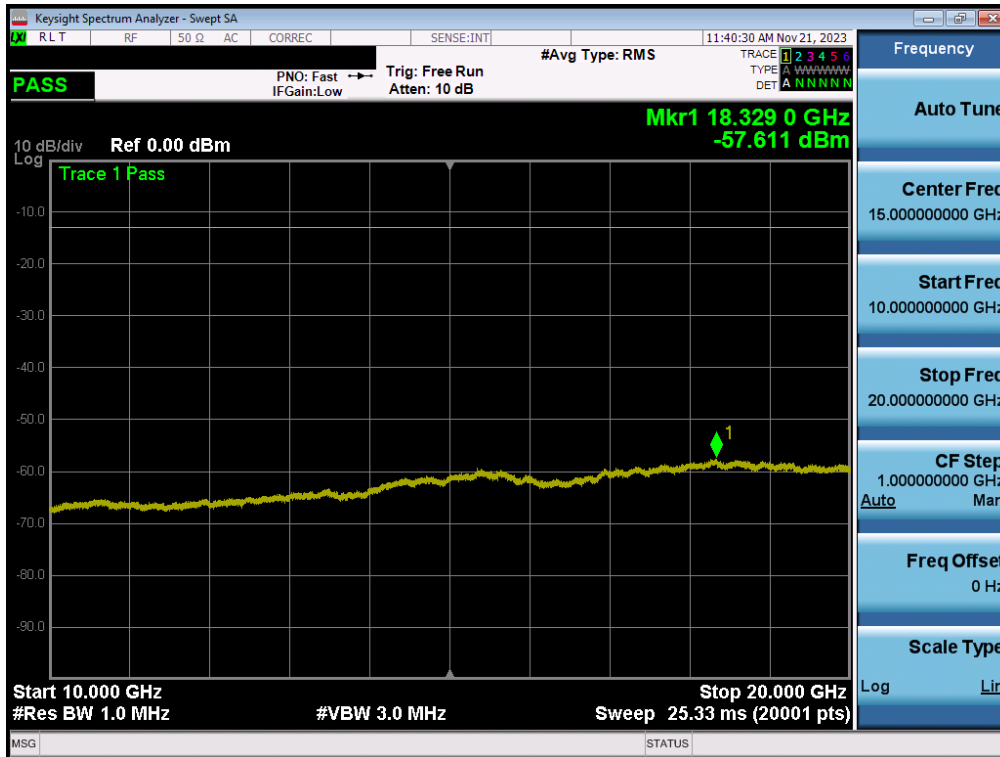
Plot 7-92. Conducted Spurious Plot (WCDMA Ch. 9538)
