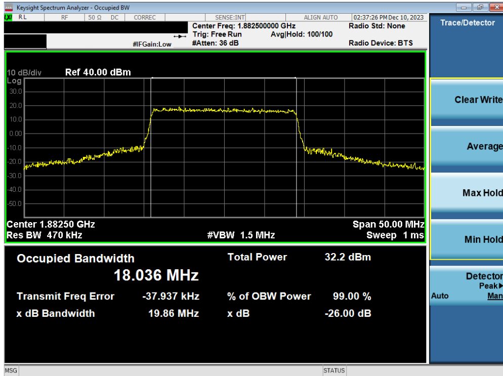
Plot 7-22. Occupied Bandwidth Plot (LTE Band 25/2 - 20MHz 16-QAM - Full RB Configuration)
