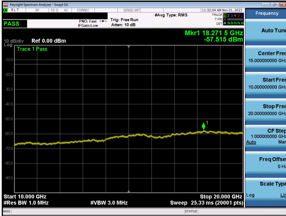
Plot 7-86. Conducted Spurious Plot (WCDMA Ch. 9262)
