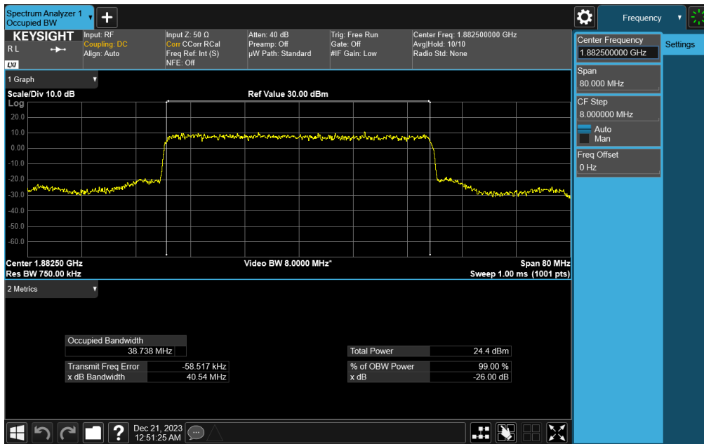
Plot 7-60. Occupied Bandwidth Plot (NR Band n25 - 40MHz DFT-s-OFDM \pi/2 BPSK - Full RB)
