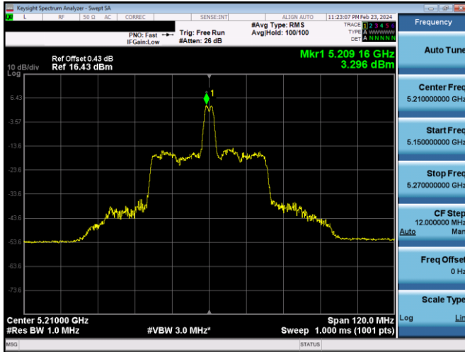
Plot 7-654. ISPD PSD SDM Diversity Antenna 4a (80MHz BW 11ax Index 18 - RU26 - Ch.42)
