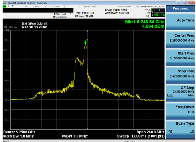
Plot 7-663. ISED PSD SDM Diversity Antenna 2a (160MHz BW 11ax Index 52 - RU52 - Ch.50(L))
