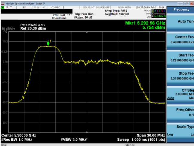
Plot 7-556. PSD CDD Diversity Antenna 4a (20MHz BW 11ax Index 37 - RU52 - Ch.60)
