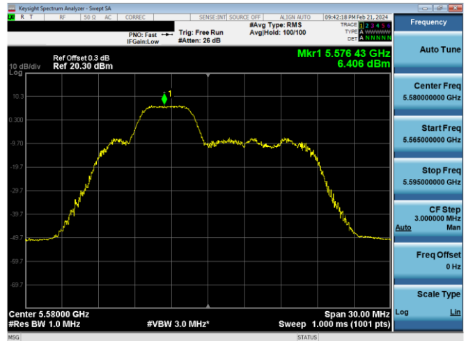
Plot 7-441. PSD CDD Primary Antenna 4a (20MHz BW 11ax Index 38 - RU52 - Ch.116)
