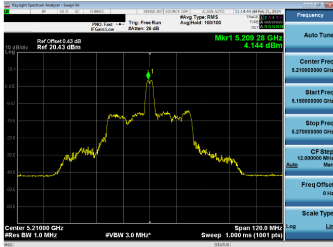
Plot 7-400. PSD CDD Primary Antenna WF5B (80MHz BW 11ax Index 18 - RU26 - Ch.42)
