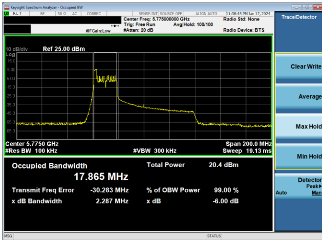
Plot 7-141. 6dB BW & 99% OBW Antenna WF5B (80MHz BW 11ax Index 0 – RU26 – Ch.155)
