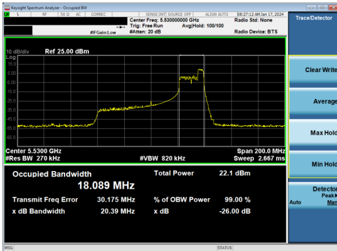
Plot 7-127. 26dB BW & 99% OBW Antenna 2a (80MHz BW 11ax Index 52 – RU52 – Ch.106)
