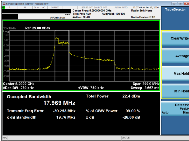
Plot 7-113. 26dB BW & 99% OBW Antenna 2a (80MHz BW 11ax Index 37 – RU52 – Ch.58)
