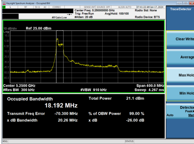
Plot 7-101. 26dB BW & 99% OBW Antenna 2a (160MHz BW 11ax Index 37 – RU52 – Ch.50 (L))
