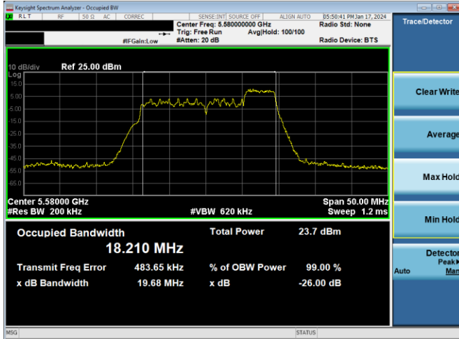
Plot 7-75. 26dB BW & 99% OBW Antenna 4a (20MHz BW 11ax Index 40 – RU52 – Ch.116)
