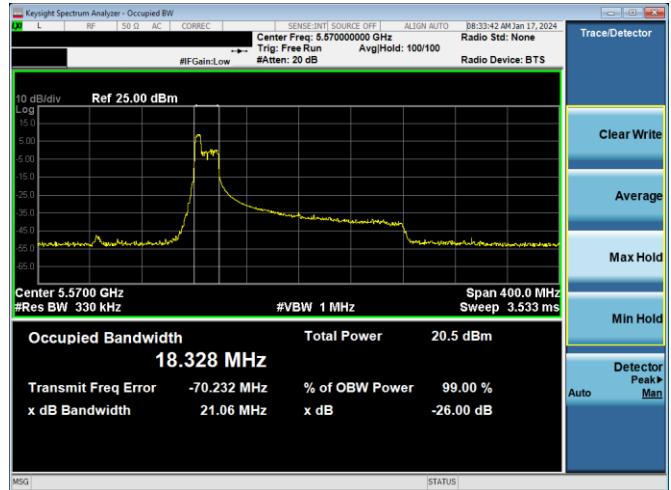
Plot 7-129. 26dB BW & 99% OBW Antenna 2a (160MHz BW 11ax Index 37 – RU52 – Ch.114 (L))
