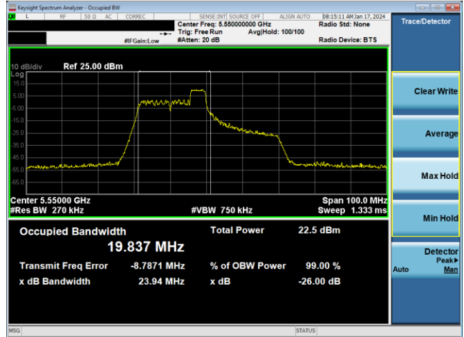
Plot 7-122. 26dB BW & 99% OBW Antenna 2a (40MHz BW 11ax Index 40 – RU52 – Ch.110)
