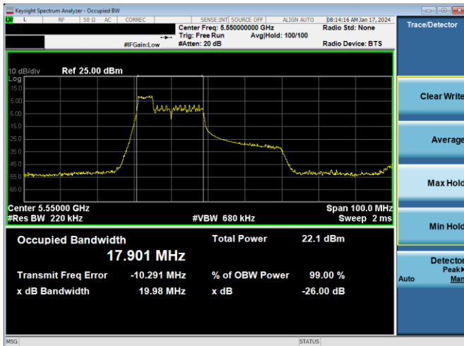
Plot 7-121. 26dB BW & 99% OBW Antenna 2a (40MHz BW 11ax Index 37 – RU52 – Ch.110)
