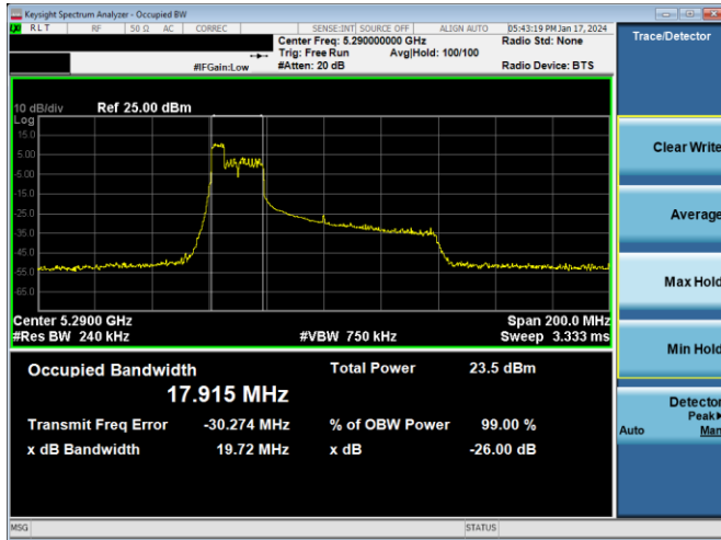
Plot 7-69. 26dB BW & 99% OBW Antenna 4a (80MHz BW 11ax Index 37 – RU52 – Ch.58)
