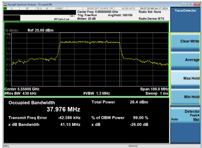
Plot 7-124. 26dB BW & 99% OBW Antenna 2a (40MHz BW 11ax – RU484 – Ch.110)
