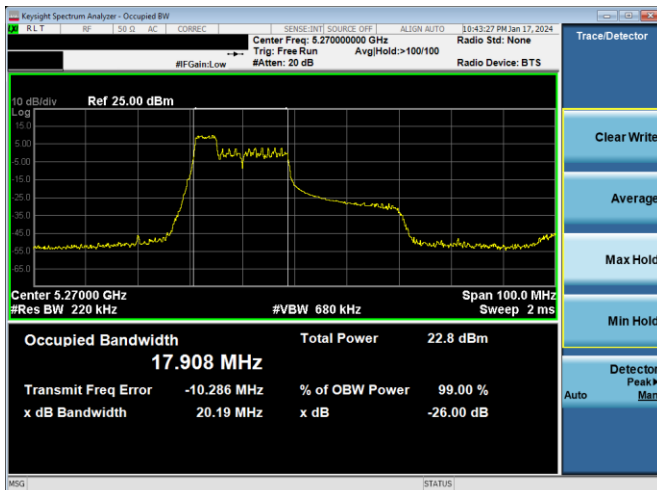
Plot 7-21. 26dB BW & 99% OBW Antenna WF5B (40MHz BW 11ax Index 37 – RU52 – Ch.54)
