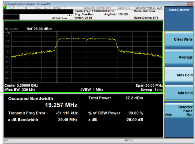
Plot 7-4. 26dB BW & 99% OBW Antenna WF5B (20MHz BW 11ax– RU242 – Ch.40)
