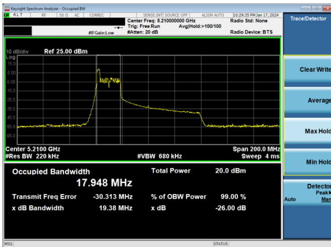
Plot 7-9. 26dB BW & 99% OBW Antenna WF5B (80MHz BW 11ax Index 0 – RU26 – Ch.42)
