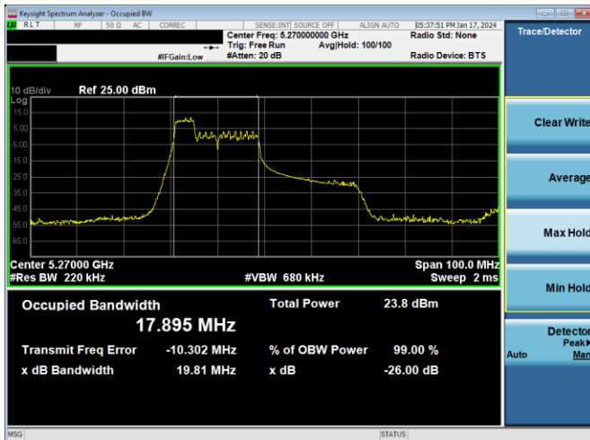
Plot 7-65. 26dB BW & 99% OBW Antenna 4a (40MHz BW 11ax Index 37 – RU52 – Ch.54)
