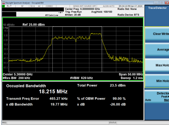
Plot 7-63. 26dB BW & 99% OBW Antenna 4a (20MHz BW 11ax Index 40 – RU52 – Ch.60)
