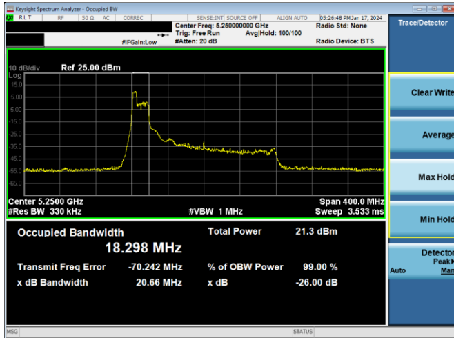
Plot 7-57. 26dB BW & 99% OBW Antenna 4a (160MHz BW 11ax Index 37 – RU52 – Ch.50 (L))
