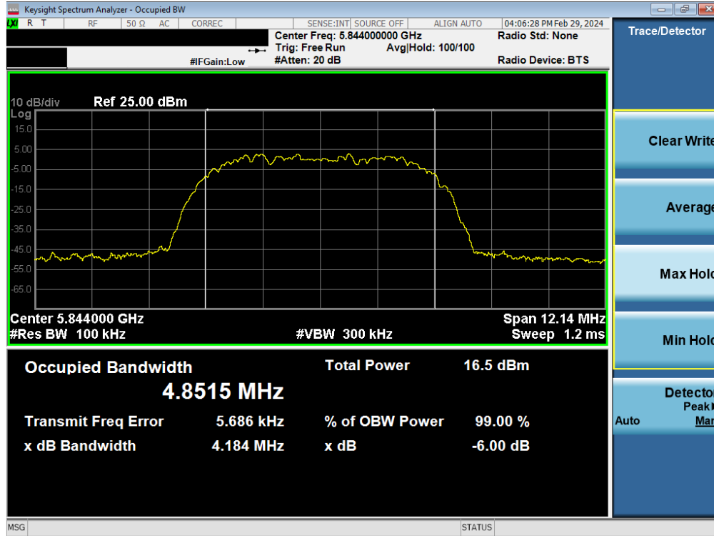
Plot 7-36. 6dB BW & 99% OBW Antenna 2a (HDR8, ePA, 5844MHz)
