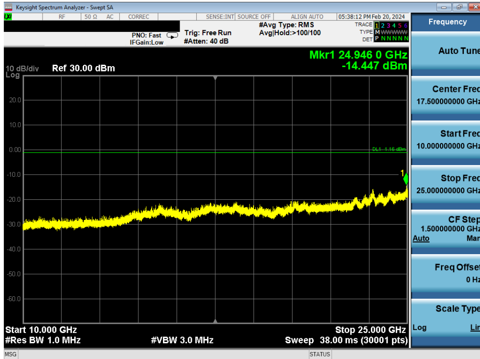
Plot 7-380. Conducted Spurious Plot Antenna 2a (802.11b – Ch. 1)
