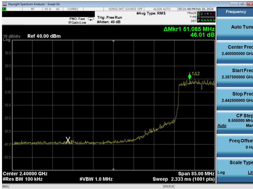
Plot 7-365. Band Edge Plot Antenna 2a (802.11ax (SU - 2.4GHz) – Ch. 6 (low)) – MCS9
