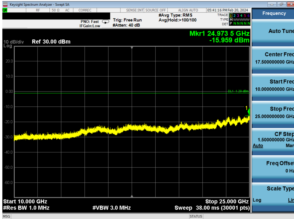
Plot 7-384. Conducted Spurious Plot Antenna 2a (802.11b – Ch. 11)
