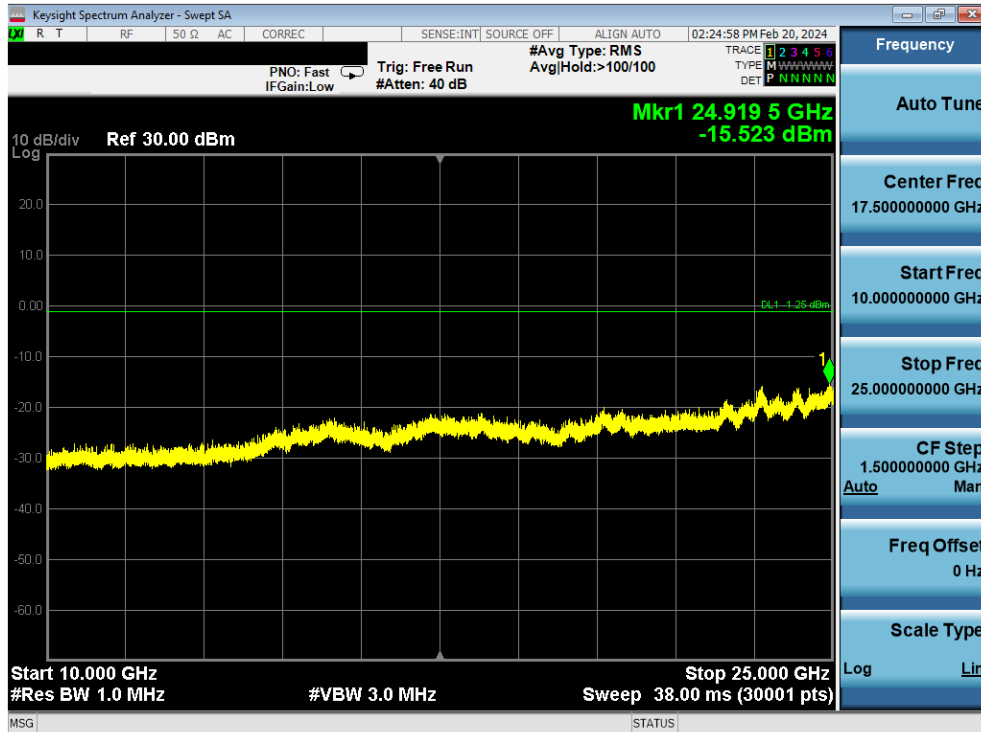
Plot 7-376. Conducted Spurious Plot Antenna 4a (802.11b - Ch. 6)
