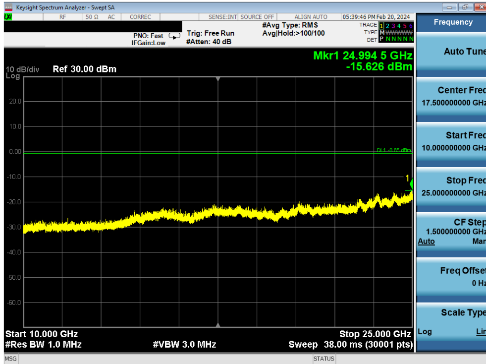
Plot 7-382. Conducted Spurious Plot Antenna 2a (802.11b – Ch. 6)
