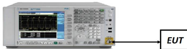
Figure 7-3. Test Instrument & Measurement Setup
