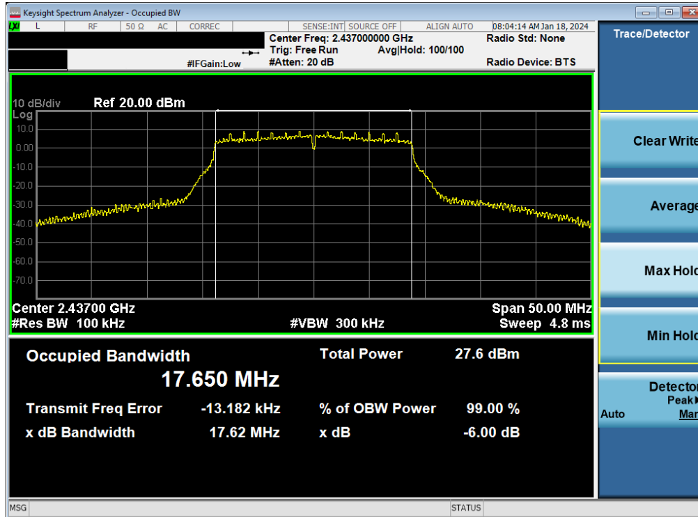
Plot 7-5. 6 dB BW and 99% OBW Plot Antenna 4a (802.11n (2.4GHz) – Ch. 6) – MCS2
