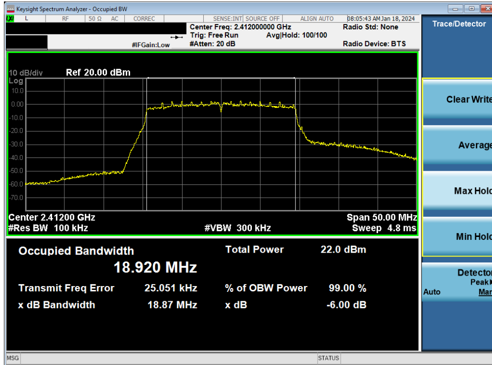
Plot 7-7. 6 dB BW and 99% OBW Plot Antenna 4a (802.11ax (SU - 2.4GHz) – Ch. 1) – MCS2
