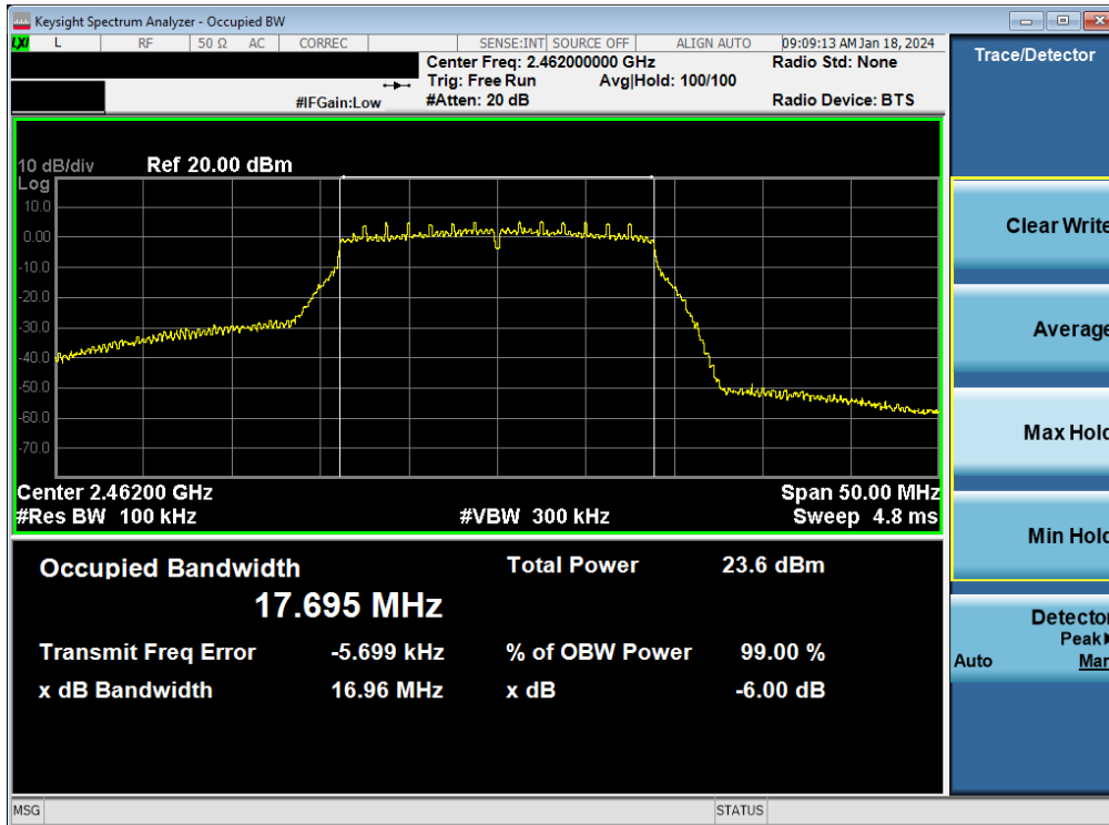
Plot 7-36. 6 dB BW and 99% OBW Plot Antenna 2a (802.11n (2.4GHz) – Ch. 11) – MCS2
