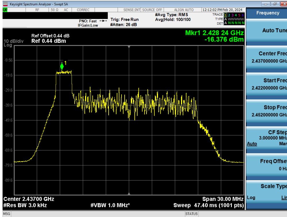
Plot 7-55. Power Spectral Density Plot Antenna 4a (802.11ax OFDMA – RU26 Index 0 – Ch. 6)
