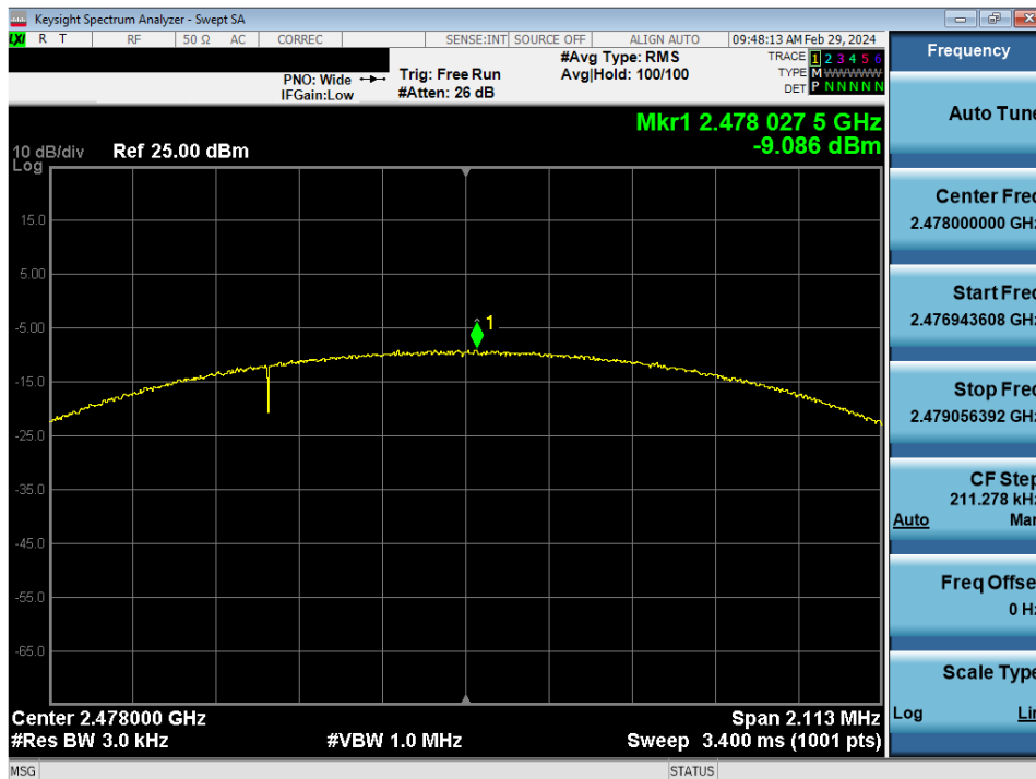
Plot 7-54. Power Spectral Density Plot Antenna 2a (Bluetooth (LE), 2Mbps, ePA – Ch. 38)
