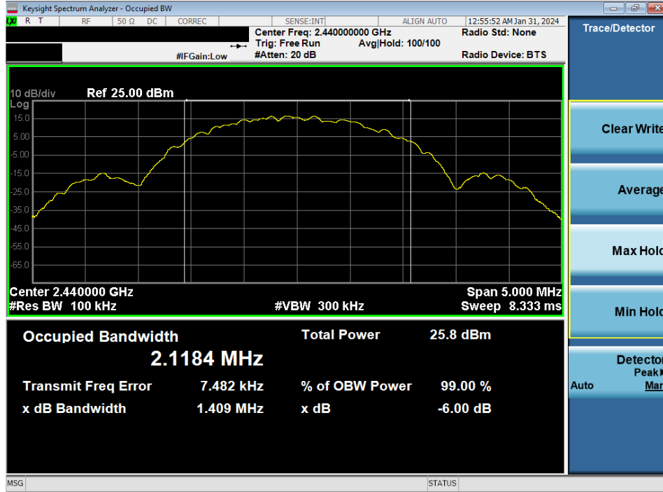
Plot 7-11. 6dB BW & 99% OBW Plot Antenna 2a (Bluetooth (LE), 2Mbps, ePA – Ch. 19)
