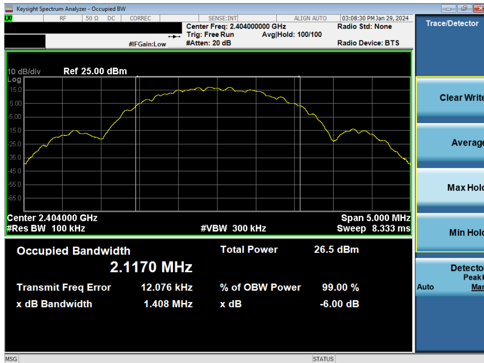
Plot 7-4. 6dB BW & 99% OBW Plot Antenna 4a (Bluetooth (LE), 2Mbps, ePA – Ch. 1)
