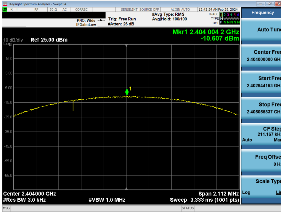
Plot 7-19. Power Spectral Density Plot Antenna 4a (Bluetooth (LE), 2Mbps, ePA – Ch. 1)
