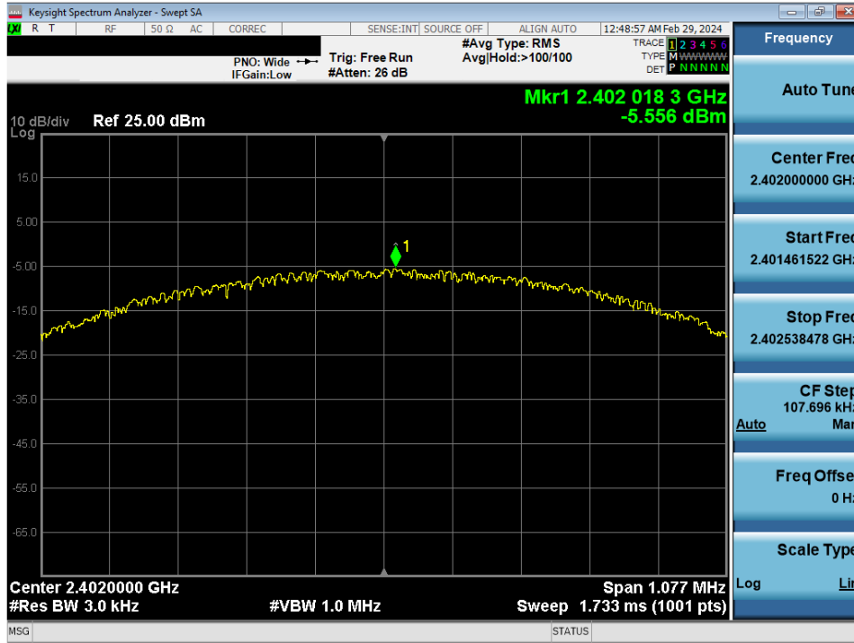
Plot 7-37. Power Spectral Density Plot Antenna 4a (Bluetooth (LE), 1Mbps, ePA – Ch. 0)
