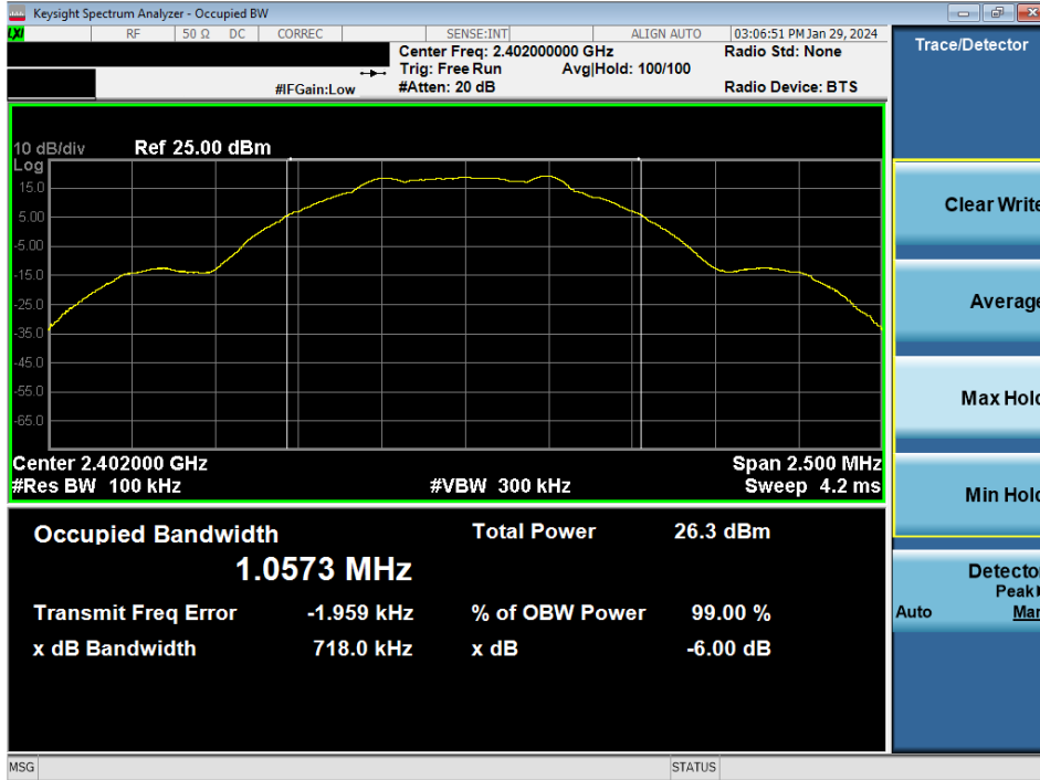
Plot 7-1. 6dB BW & 99% OBW Plot Antenna 4a (Bluetooth (LE), 1Mbps, ePA – Ch. 0)
