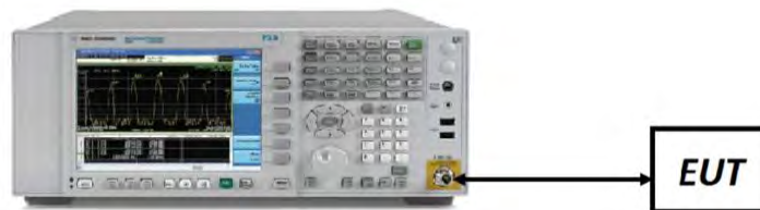
Figure 7-3. Test Instrument & Measurement Setup
