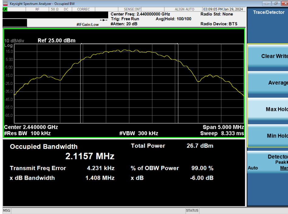
Plot 7-5. 6dB BW & 99% OBW Plot Antenna 4a (Bluetooth (LE), 2Mbps, ePA – Ch. 19)
