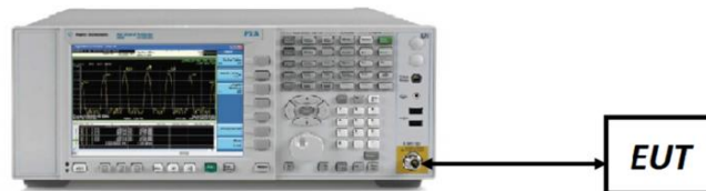
Figure 7-5. Test Instrument & Measurement Setup
